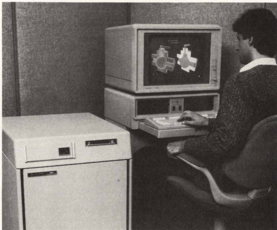
Figure 1: The Harris 60 superminicomputer supports multiple CAE graphic display systems and other design peripheral equipment.
