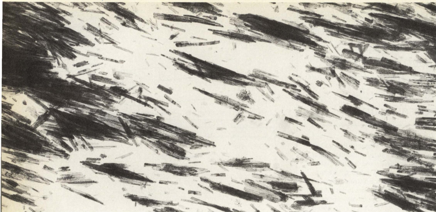
Figure 2: The bias of standard magnetic particles is obvious in this 42,050 times magnification from 3M.
