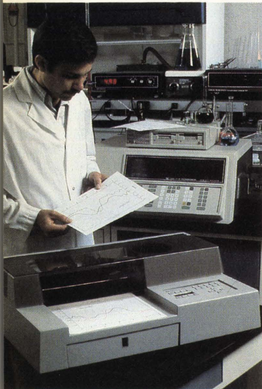
Figure 3: The Hewlett-Packard 7550A may be the first plotter to break the 4G acceleration standard.
