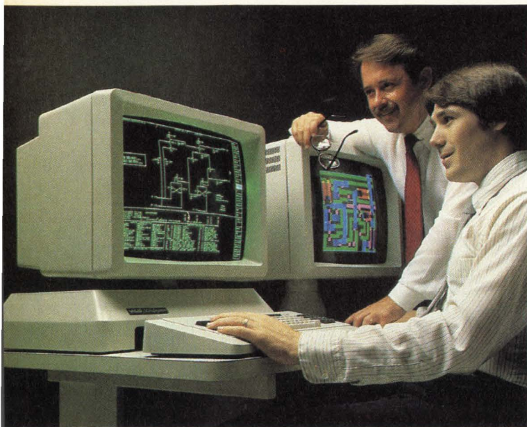
Figure 7: The SCALDstar integrated VLSI logic and layout design system for custom and semi-custom design.
