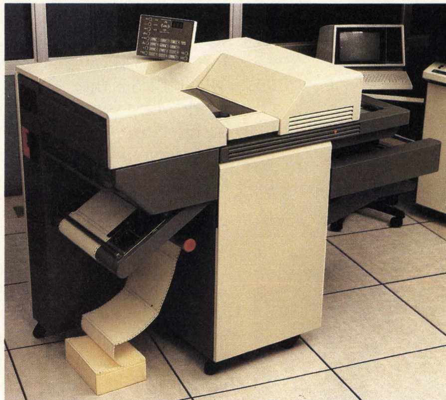
The MP6090 uses magnetic perpendicular printing with a 100 mm diameter magnetic drum rotating at a constant speed of 12.5 in/sec.
