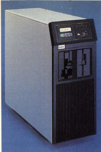
Figure 5: A microprocessor-based multiuser system from Callan Data Systems that utilizes memory management, cache, communications, and I/O support.
