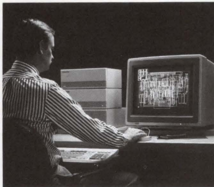
The 300,000-vector/sec graphics-performance rate offered by the HP 9000 Model 350CHX translates to a reaction time of approximately 0.25 sec in applications such as pc-board design.
