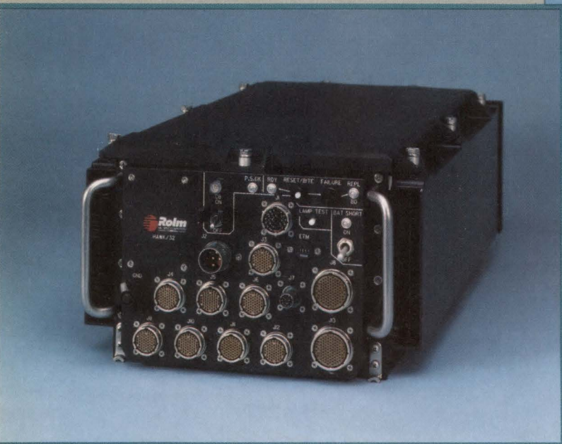
MIL-spec (left) and ruggedized (above) versions of the Data General MV 8000 Series computer (Rolm Mil-Spec Computers)
