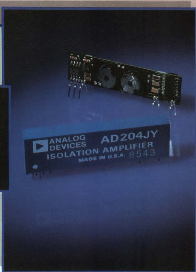
1500V rms, 2-in.-long x 1/4-in.-wide IA (Analog Devices Inc)
