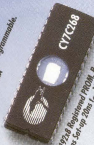
C17C255 2048x8 Registered PROM. Reprogrammable. 18ns Set-up 12ns t co 120mA
