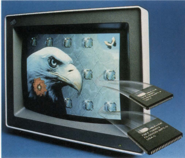
The VGA standard supports analog monitors; the VGA-compatible chip set from Cirrus Logic lets you display as many as 256 colors with more subtle shading than is possible using the EGA graphics standard and a digital monitor.
