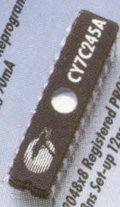
C17C245 2048x8 Registered PROM. Reprogrammable. 25ns Set-up 12ns t co 90mA
