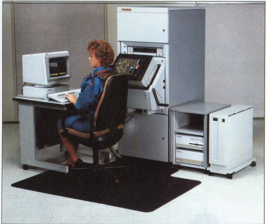
This board test system, Hewlett-Packard's 3065ST, performs digital in-circuit and analog-functional tests. An automatic program generator for it runs on the vendor's workstations.
