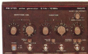
PM 5705 Pulse Generator. 0.1 Hz to 10 MHz; 15V output amplitude; 10 ns rise time; external triggering.
