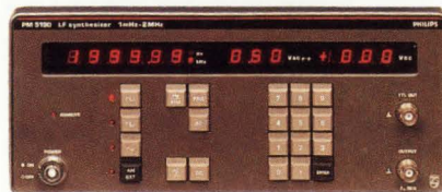
PM 5190X Synthesized Function Generator. 1 mHz to 2.147 MHz; sine, triangle, square waveforms; TTL output.
