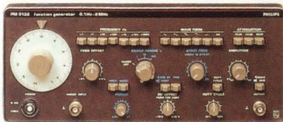
PM 5132 Function Generator. 0.1 Hz to 2 MHz; five waveforms; sweep, VCO modes; variable duty cycle.
