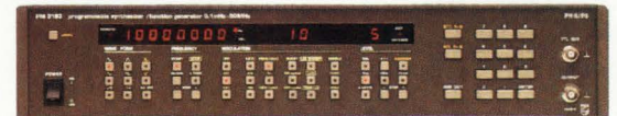
PM 5193 Programmable Synthesizer/Function Generator. 0.1 mHz to 50 MHz; full 8 digit resolution, and eight standard waveform outputs. FM, AM, GATE, SWEEP, and BURST modulation. Full IEEE-488 control.
