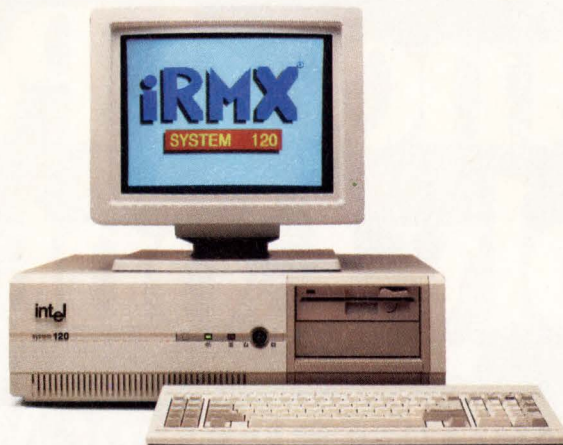
System 120. The first integrated real-time system based on the AT-bus with iRMX® software.
