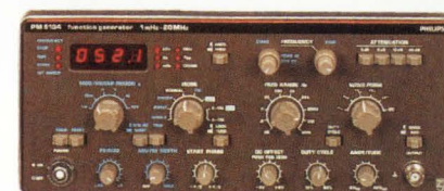
PM 5134 Function/Sweep Generator. 1 mHz to 20 MHz; five waveforms; sweep, burst, single modes; 20Vp-p output.
