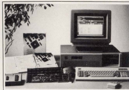
This logic design verification system handles both ASICs and PLDs, allowing you to develop test programs and perform functional tests on your design.
