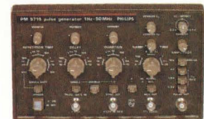
PM 5718 Pulse Generator. 1 Hz to 50 MHz; 6 ns to 500 ms rise/fall times, 10V amplitude.
