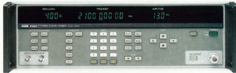
6062A Synthesized RF Signal Generator. 100 kHz to 2100 MHz frequency output range, with \pm 1 dB amplitude accuracy to 1 GHz, \pm 1.5 dB to 2.1 GHz. Includes amplitude, frequency, phase and pulse modulation. Featured is a fast-rise 15 ns pulse modulator using gallium arsenide technology. IEEE-488 is standard.
