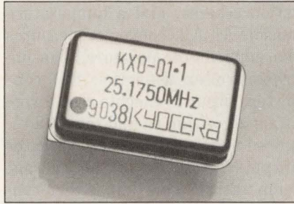
Housed in all-metal DIPs, KXO-01 crystal oscillators from AVX/Kyocera output frequencies of 4 to 50 MHz. They meet FCC EMI specifications and feature a \pm 100 -ppm stability from 0 to 70°C.
