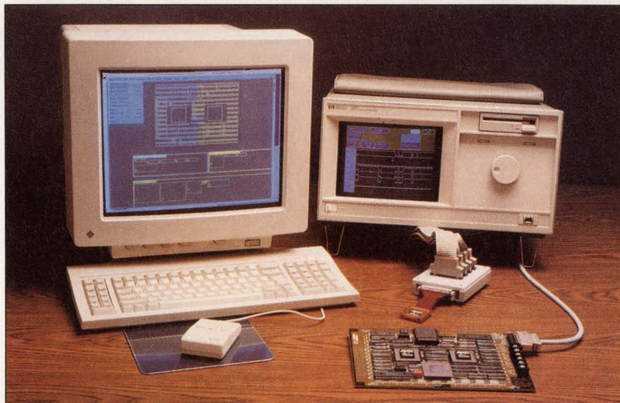
Chip, board, and software products together provide field-programmable interconnections for circuit boards. Prototype construction may never be the same.
