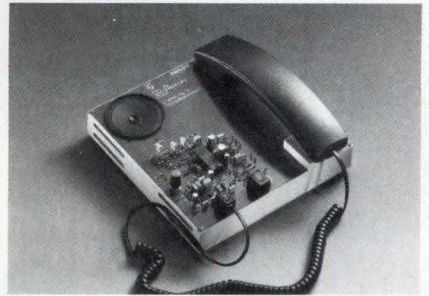
The TEA1096 and TEA1096A offer highly integrated single-chip solutions to all the speech, transmission, listening-in and line monitoring functions required in modern line-powered featurephones.
