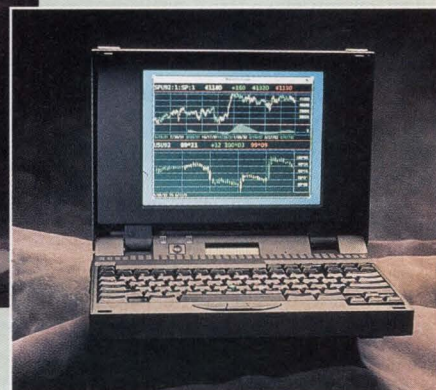
Tadpole's 6-lb SPARCbook 3 portable workstation delivers 26 SPECint92 and 21 SPECfp92 and costs $7500 to $10,000.
