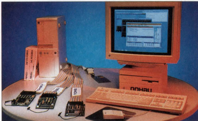
The LanICE (box on the left) contains as many as five ICEs. It allows you to control the ICEs from a networked workstation running X Windows.
