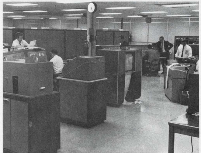
Layout of center must conform to predetermined pattern with one-third of an inch to avoid losses and cross talk in connecting cables. The method of redundancy through switching rather than by means of more equipment results in more wiring and cables than usual.
