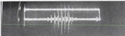
Response of a faulty CW oscillator, causing it to squibulate, or produce side bands around the fundamental signal.
