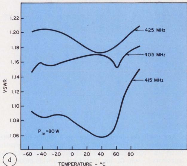
4. Measured results of the multiplier design reveal a linear input/output power variation (a) and a 1-dB bandwidth of 14% (b). Operation up to a base-plate temperature of 80 C is possible (c), while VSWR over the -60 to 90 C range is held below 1.22:1.
