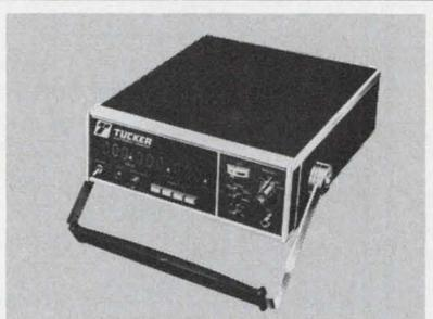
**Tucker 550 MHz Frequency Counter.** 9 full digits with a resolution of 1Hz the Tucker 5509 Counter is a tiny, low-cost and simple to operate Counter. Aging Rate is  $1 \times 10^{-6}$ /day. Price \$950. Send for free catalog. Tucker Electronics Company, P. O. Box 1050, Garland, Texas. (214) 348-8800.
