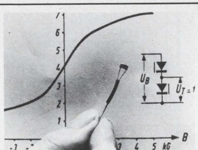
**EPP AHY10 MAGNETIC DIODES** change internal resistance as function of external magnetic field. AHY10A passes 1mA at BV with sensitivity of 0.75 — 1.0V/kG. Four types. Numerous uses. 8-page application note, full data available: European Electronic Products, 10180 W. Jefferson, Culver City, Ca. 90230 213/838-1912
