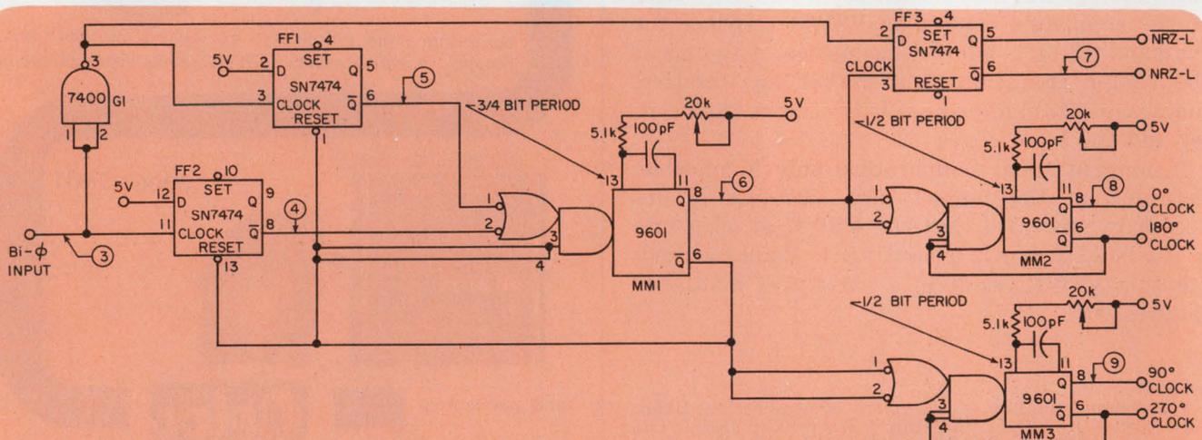
1. Flip-flop FF<sub>3</sub> provides an NRZ-L output, and MM<sub>2</sub> yields a clock in phase with the NRZ-L signal
