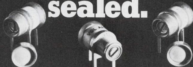
The capless design of Voltronics "A" line eliminates many problems such as moisture and dust penetration and lost caps that traditionally plague conventional air trimmers. Permanent sealing is achieved in our white room with an "O" ring that will withstand 40 p.s.i. Another plus is smooth linear tuning (see curve) due to its non-rotating design with twice the resolu-
