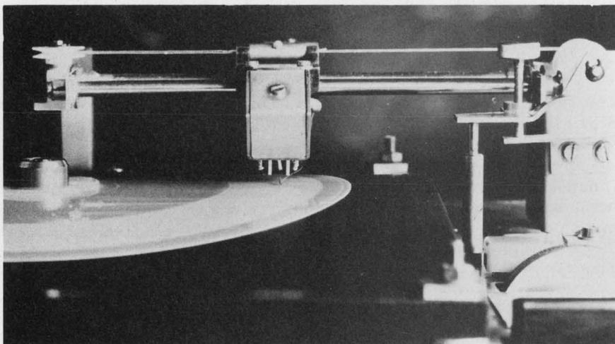
A thin plastic disc coated with foil spins at 1500 rpm in making video hill-and-dale recordings in Teledec's system. Single-disc players and automatic changers with two hours playing time are under development.
