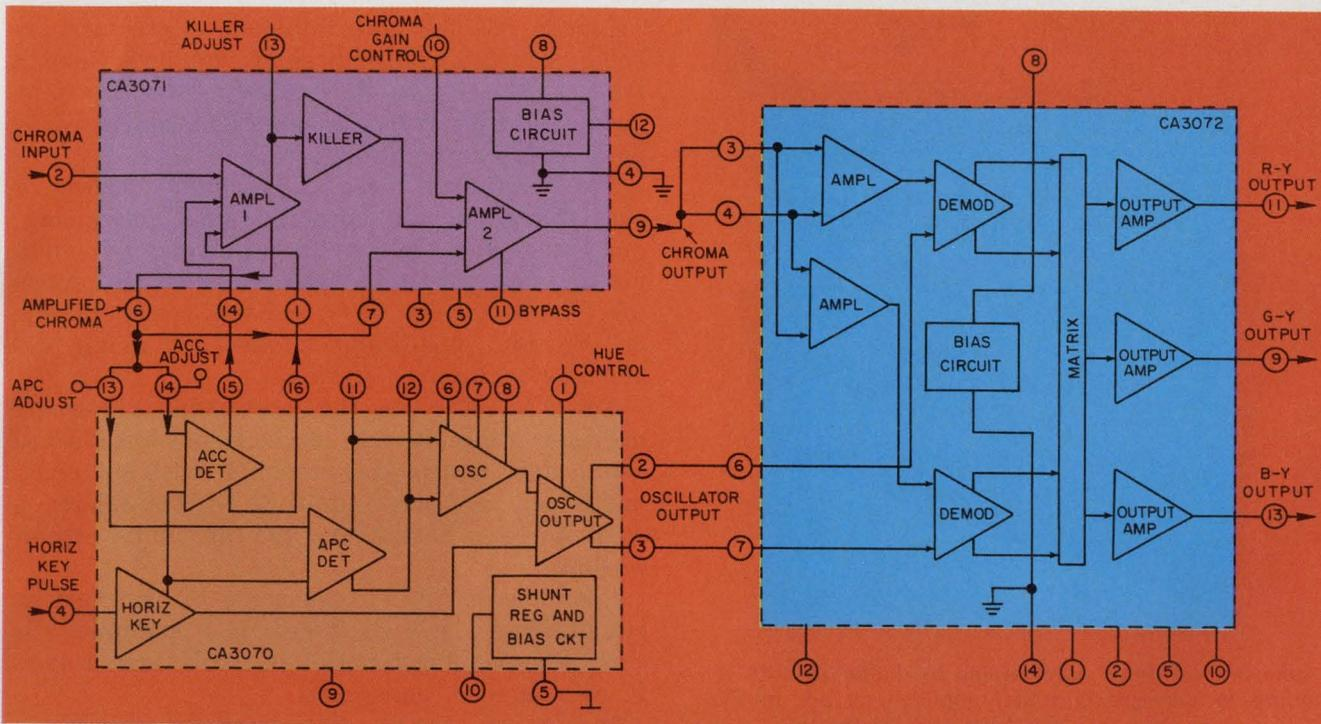
A complete chroma system for high-quality television receivers, by RCA, comprises three IC packages. The IC at bottom left is a complete subcarrier regeneration system.
