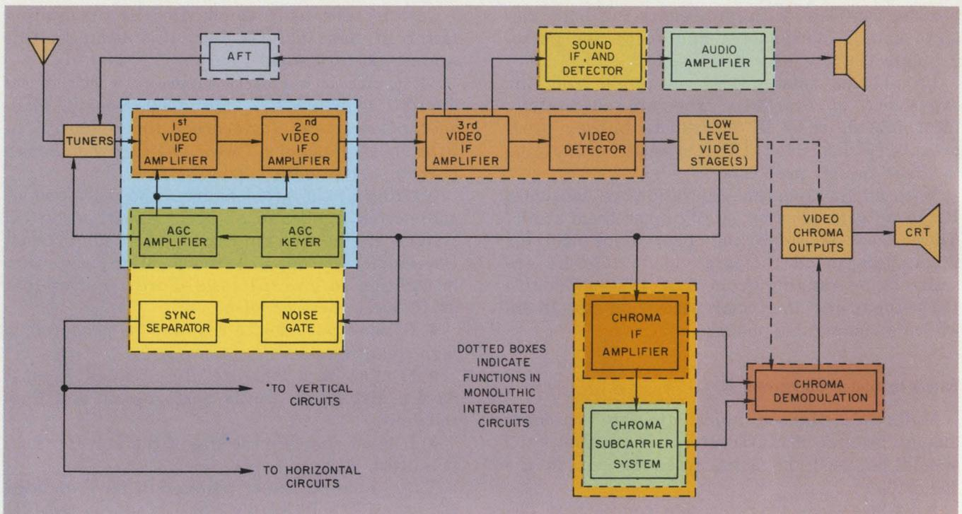
ICs are being used in color television receivers to perform several subsystem functions. The ICs, indicated by dotted boxes, can provide complex circuits and better
