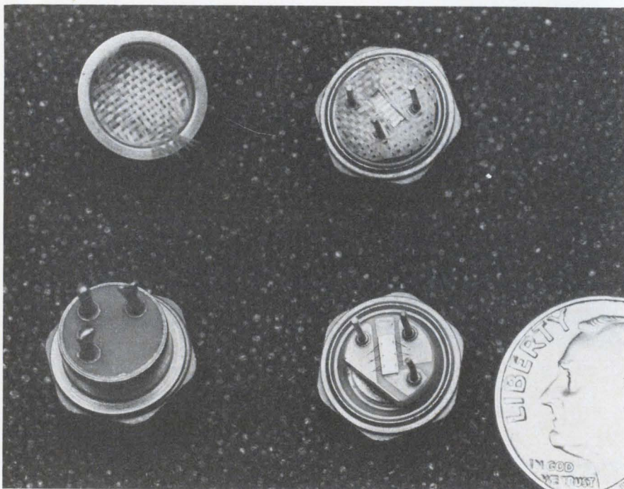
Heat pipes for transistors are fabricated with Refrasil fiberglass wick structures. Here a 2N5701 transistor on a TO-60 header is in various stages of assembly. The sealed transistor is filled with 3M FC-77 fluid.
