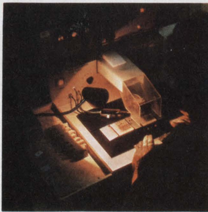
Abrasive trimming is frequently used to trim thick-film resistors at Raytheon's hybrid-facility, especially where stability is a prime concern.
