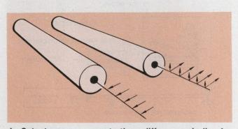
4. **Output-power concentration differs markedly** for polarized and unpolarized lasers. In a linearly polarized laser (left), power concentrates in a single plane. An unpolarized unit distributes most of the power between two orthogonal planes.
