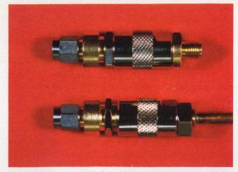
A connector with a built-in line stretcher is the Phase Adjustable SMA from Amphenol. The connector comes either as an individual component or as a cable terminator. VSWR is better than 1.28:1 up through 18 GHz, and the phase can be adjusted by 10° times the frequency in GHz. Thus, at 10 GHz, the phase can be adjusted up to 100°.
