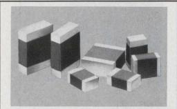
HIGH Q MULTILAYER CAPACITORS feature very high quality factors at microwave frequencies. Offered in three standard sizes: .050 x .040, .080 x .050, .125 x .095. Capacitance values from 0.1 pf to 1000 pf with close tolerance and voltages to 1000 VDCW. Johanson/Monolithic Dielectrics Div., Box 6456, Burbank, Ca. 91510, (213) 848-4465.
