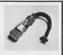
HORN ANTENNA ... I/J Band, circularly polarized, octave bandwidth, fan beam, 500 W CW, WRD750 WG input and a sampling probe. ECM application. Part shown with a pressure window and flexible WG.
