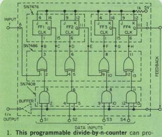
vide symmetrical outputs with the use of only conventional digital ICs. changes state, all flip-flop inputs programmed with a ONE also change their phases. This action is delayed by time t, which results from the combined switching delays of the flip-flops and gates in the signal path. Note the phase changes in the waveforms between E and F, C and D, and A and B where  $S_1$ ,  $S_2$  and  $S_3 = 1$ . The phase between G and H doesn't change;  $S_4 = 0$ . The resulting output I is symmetrical.
