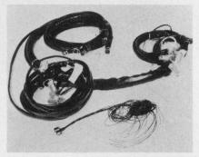
Fiber-optic coupling interface for Naval aircraft offers significant size and weight reduction over point-topoint wire cabling.
