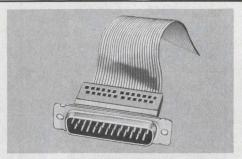
**AMPLIMITE HDF CONNECTOR** mass-terminates quickly, at low cost. Accommodates solid or stranded round-conductor flexible cable on .050" centers. Forks penetrate cable from opposite sides, trap each conductor, then interlock with housing. Pin and socket contacts intermateable with industry standards. From the people who offer you technical assistance: AMP Incorporated, Harrisburg, Pa. (717) 564-0100.
