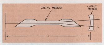
1. A laser is actually a resonant cavity that can support oscillations at light frequencies. The cavity's lasing medium provides gain, while the mirrors at each end provide feedback. A slightly transparent mirror serves as the cavity's output.
