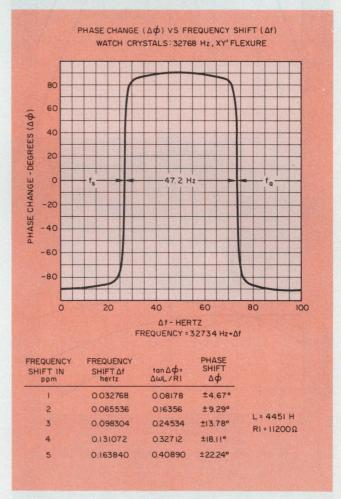
4. The phase of a signal passing through a crystal changes sharply from -90 to +90 degrees as it passes through its series-resonant frequency,  $f_s$ . It changes from +90 to -90 at its anti-resonant frequency,  $f_a$ . The higher the Q, the sharper the change.
