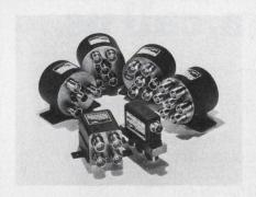
**COAXIAL SWITCHES**, Type DX, MX and HX are designed for high average power up to 6.5 GHz; example: 1500 watts at 1 GHz All actuators are 28 Vdc, fail-safe for SPDT and Transfer, selective for multi-throw. All have type SC connectors.
