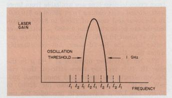
3. Slight variations in the length of short laser cavities can cause more than one longitudinal mode to propagate, thereby affecting power and polarization.
