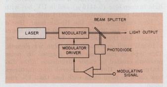
2. A feedback modulation scheme cancels low-frequency noise, eliminates drift and linearizes the modulator.
