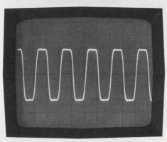
Unretouched scope display of the 3312A's 10 MHz square-wave output, showing 18 nsec rise time.
