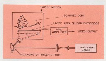
6. Facsimile equipment employs a laser-based flyingspot scanner. High-resolution laser light scans an image a line at a time, while a photodiode detector picks up the intensity-modulated signal. The image, or scanned copy, moves vertically.
