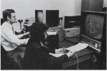
**Updated information** is being entered into the CEEFAX system via computer terminal (upper left), while a TV monitor shows a weather map that is being transmitted (lower right).
