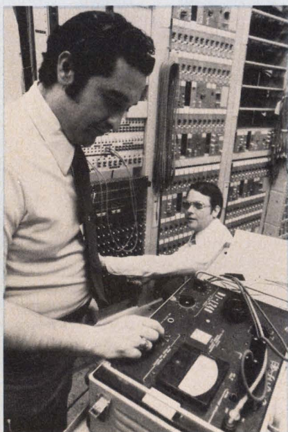
A digital system to use the gaps in voice communication is being tested for domestic telephone use.
