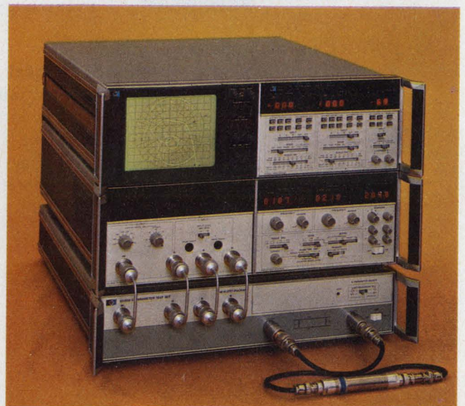
Add an S-parameter test set to a network analyzer and you can measure transistor forward and reverse gains or input/output impedances (Hewlett-Packard).
