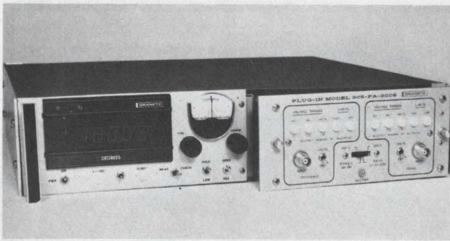
Digital readout of gain, phase and amplitude mark the Series 305, from Dranetz Engineering Laboratories. The autoranging unit works to 700 MHz.
