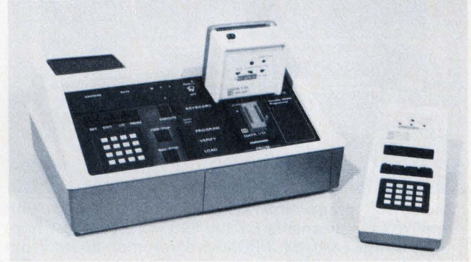
Complete with a portable RAM-pak, DATA I/O's Model IX programmer can program or emulate any type of bipolar PROM array available.
