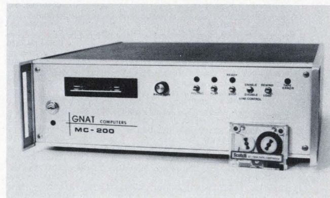
Hardware and software control 3M's DCD-100 mini-cartridge drive in Gnat Computers' \mu P-based MC-200.
