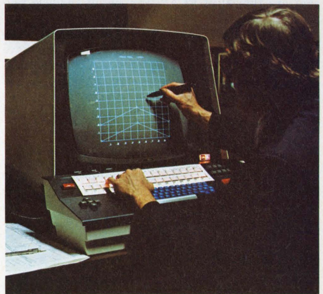
When you design circuits with a computer, you can change the performance with the stroke of a pen, as on this Sanders console. The computer may even display the revised schematic.
