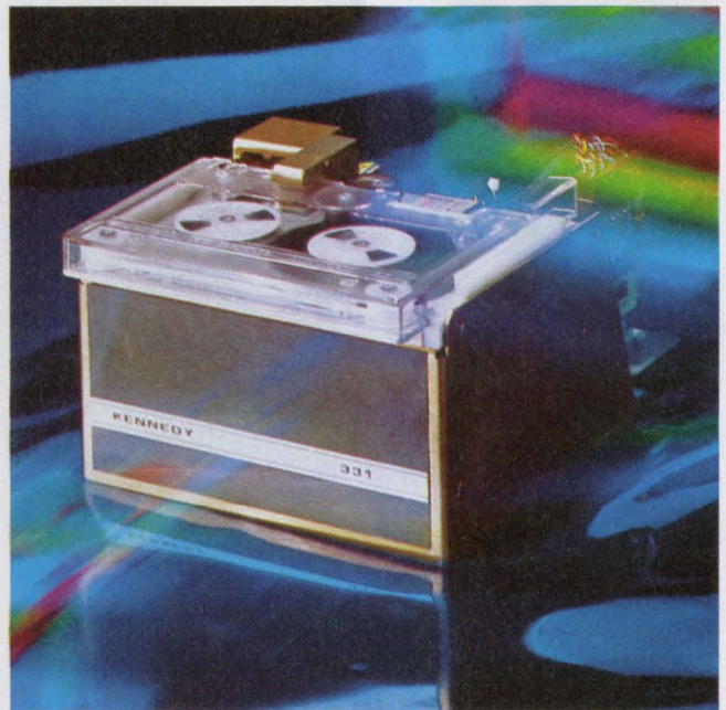
The DC-300 cartridge is electromechanically locked into Kennedy Co.'s Model 331 drive, until its release by an Unload command. All four of the serially sequential tracks can be accessed without turning the tape.
