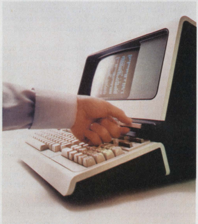
Forms are retrieved selectively in seconds from the mini-cartridge storage in Hewlett-Packard's 2644A Mini Data Station. The terminal uses HP's own drive, which is not yet available by itself.
