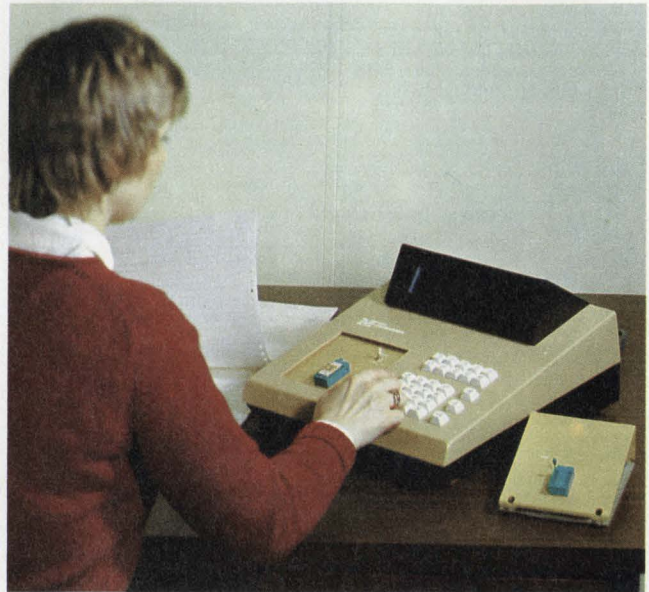
Able to program any bipolar or MOS PROM, the IM1000 programmer from International Microsystems includes a TTY interface as well as two RS-232 ports as standard.
