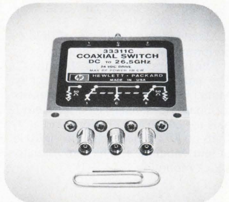
Internally switched 50Ω loads in this SPDT switch provide all-matched ports to 26.5 GHz.
