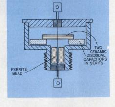
a dc resistance of less than 6 m $\Omega$ . The filter can have a 0.375-in. diameter and is fitted with a ¼-28 threaded mounting stud.
