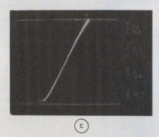
1. Conventional planar SCRs (a) aren't suitable for ICs. Harris' dielectric isolation prevents diffused SCRs from interacting with the substrate (b). A DI SCR's forward voltage with both gates floating is fairly linear when plotted vs current (c).
