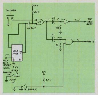
4. **Memory-write control is simple** and straightforward. When the write-enable switch is closed, pressing the Inc-Mem button will generate first a write pulse (through  $C_1R_1$ ), then a positive edge to increment the memory address through  $C_2R_2$ .
