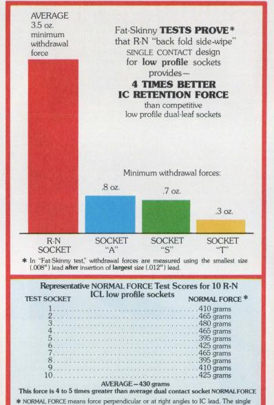
ICL contact exerts this kind of force against the IC lead when inserted into the socket.
