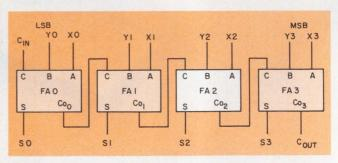
2. Four-bit, ripple-carry full adders are slow because carries from LSB to MSB take time to ripple through.
