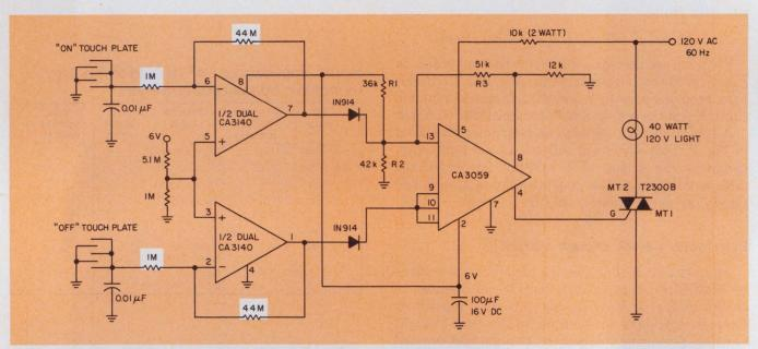
4. The op amp's high input impedance allows 1-M $\Omega$  input resistors to be used in this nonmechanical switch. These
