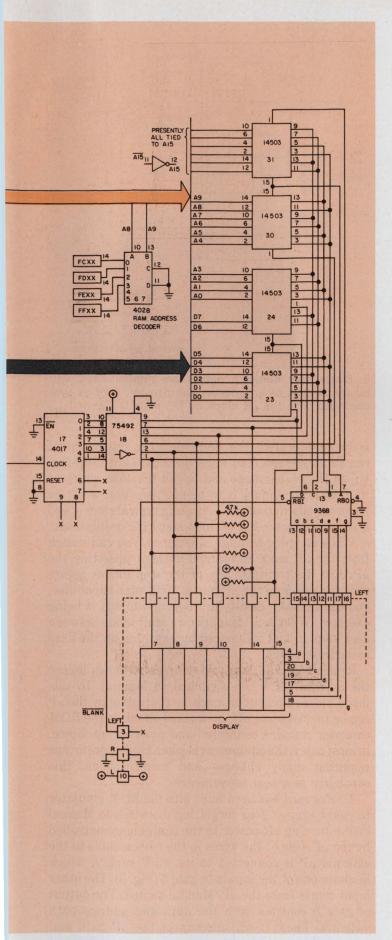
3. Thirty chips and a few other components are all that's needed to build a complete ROM emulator, or development system for a microprocessor.
