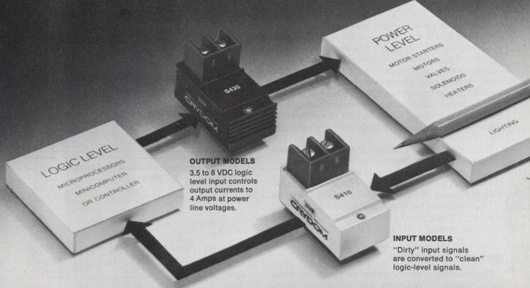
AC and DC Solid-State Input Switches and companion Output Switches that deliver 4 Amps at 40° C, 2.75 Amps at 70° C Ambient . . . without added heat sinks.
