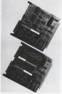
**Boards for the Zilog Z-80**  $\mu$ **C** are based on Data Translation's DATAX modules and feature analog I/O and analog-input systems.
