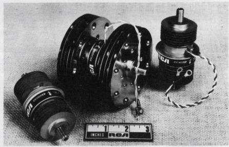
**Transcalent cooling** from RCA, which uses a heat-pipe technique to remove heat from semiconductor chips of diodes, transistors and SCRs, shrinks device sizes to as much as 1/7. A typical 16-lb assembly becomes only 10 oz. Some units handle as much as 400 A at 1200 V.
