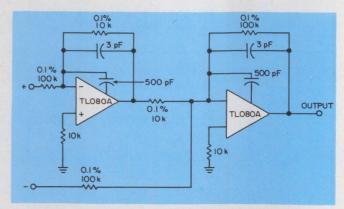
2. This instrumentation amplifier handles  $\pm 100$  V of common-mode signal. Also, the BIFETs provide a power bandwidth of 1 MHz at a gain of 10, plus the BIFET specialty —an input impedance of  $10^{12}~\Omega_{\cdot}$
