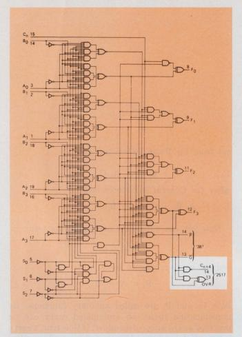
4. **Outputs determine how the Am25LS381/Am25LS2517 is used.** The highlighted portion is the Am25LS2517 configuration, which can be used for ripple-carry applications either between blocks or over block groups.
