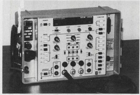
A useful combination for digital-circuit testing, frequency and transition counters, a voltmeter, and a logic probe, are built into the Data Test 1200. This one is built especially for Burroughs.
