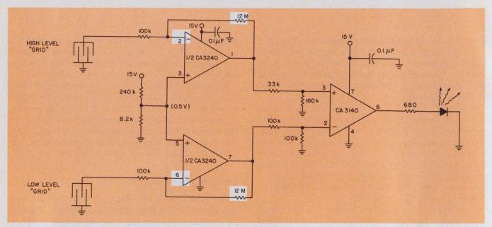
3. In a liquid-level sensing system, high feedback resistances yield the required high gain.
