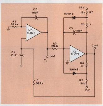
5. Stable operation at 100 kHz from this precision quadrature oscillator is due to the BIFETs. Only  $R_5$  and  $R_7$  must be trimmed for a symmetrical output.
