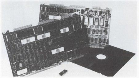
**Software operating systems can be stored** on Intel's SBC 80 single-board microcomputers internally in semiconductor ROM or externally on diskettes. This feature is possible thanks to Intel's new RMX/80 Real-Time Multi-Tasking Executive software package.
