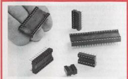
METHODE IC SOCKETS are end and side stackable for ultra-high density packaging. Sizes for all standard DIP packages are available on .300", .400" and .600" centers. Anti-wicking contact design with stand-off makes soldering and clean-up easy. Large ramped lead-in for simple assembly and field repairs. Insulators are glass filled nylon and contacts are tinplated brass. Methode Manufacturing Corp. 1700 Hicks Road, Rolling Meadows, IL 60008, (312) 392-3500.
