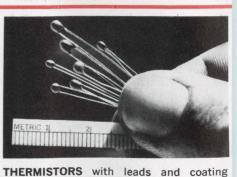
with modern circuit design. R @ 25°C  $100\Omega$  to  $1~{\rm meg}~\Omega~\pm 10\%$  to  $\pm 1\%$ . CURVE MATCHED INTERCHANGEABLES to ±.25°C. POINT MATCHED INTERCHANGE-ABLES to ±.2°C. Call or write for HP97 or TI SR52 THERMISTOR LINEARIZATION PROGRAM. WESTERN THERMISTOR CORPORATION, 354 Via Del Monte, Oceanside, CA 92054. (714) 433-4484.
