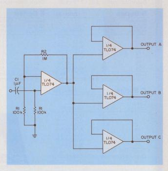
6. Process audio signals with  $100\text{-}k\Omega$  input impedance plus low distortion and noise over the full audio bandwidth, with only one BIFET quad.
