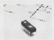
7105A offers one single-turn trimmer with one series-fixed resistor in a 6-pin DIP. Model 7107C is designed for opamp gain-trim applications. It consists of one single-turn trimmer with two series fixed resistors and one discrete fixed resistor in a 14-pin DIP.
