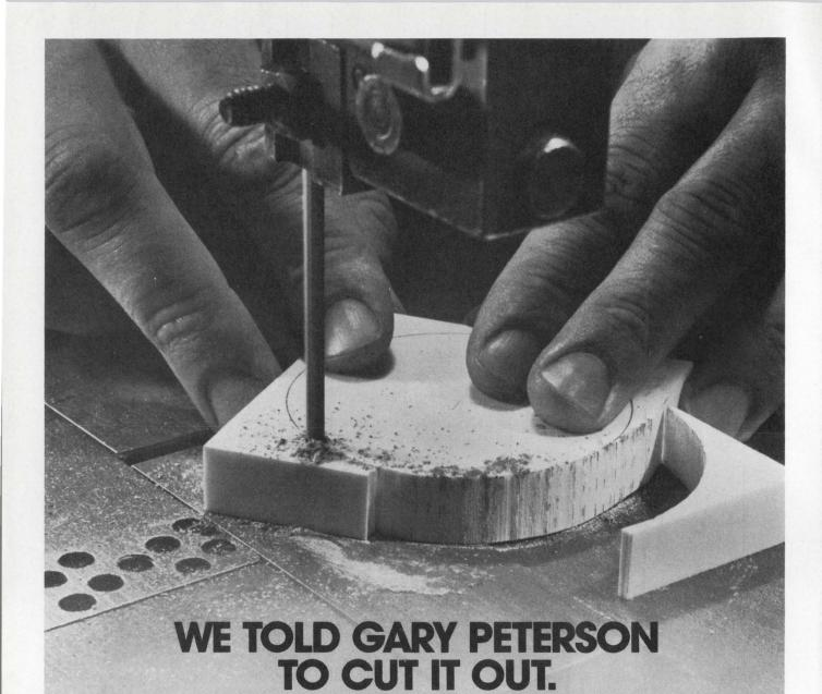
Design engineer Gary Peterson chose MACOR machinable glass-ceramic instead of alumina or beryllia for the 2½ inch diameter circuit base that is the heart of a new angle transducer manufactured by Hewlett-Packard.
