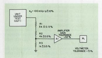
1. Only the tolerance limits of each system component are needed to establish the over-all accuracy of the readings taken in a measuring system.
