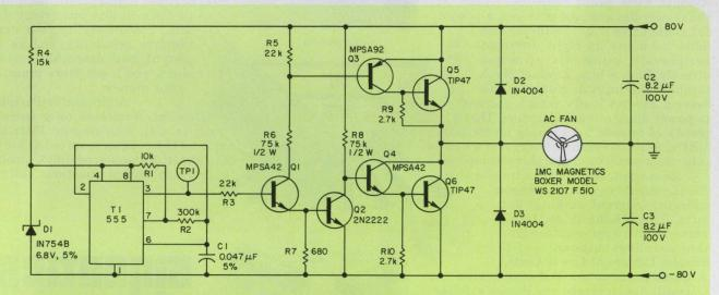
A low-cost power inverter can drive two small ac fans from a ±80-V-dc power source.
