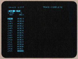
**Observing state display** shows address flow at the moment the glitch occurs and reveals that the I/O port address 8080 always accurs at the same time. This would lead you to observe I/O related signals for transitions occurring simultaneously with the glitch.
