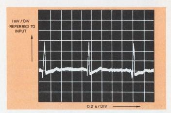
2. This electrocardiogram's low "grass" and hum levels result from matching resistors in the circuit of Fig. 1 for a high common-mode rejection ratio.
