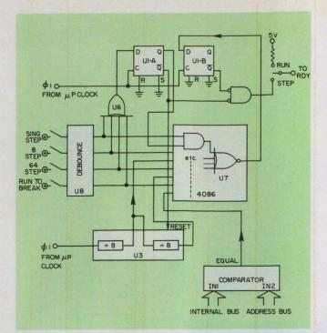
5. Single and multistep modes are implemented with binary dividers or an address comparator. Each is synchronized with the  $\mu P$  clock by flip-flops U  $_{1A}$  and U  $_{1B}$ .
