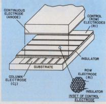
A switching point from one color to another is established by adding a control electrode so that each element is either on or off, not in between.
