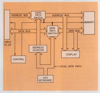
1. A simple microprocessor development system can be built quickly and inexpensively. The memory connects either to an internal keyboard or to an external  $\mu P$ . In either mode, the information on the address and data buses is displayed on a simple, calculator-like display.
