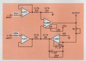
3. High resistance at the input leads doesn't generate excessive voltage offsets because of the BIFET's low input-bias current. The  $100\text{-}k\Omega$  resistors minimize input reflections from the differential inputs of this variable amp.
