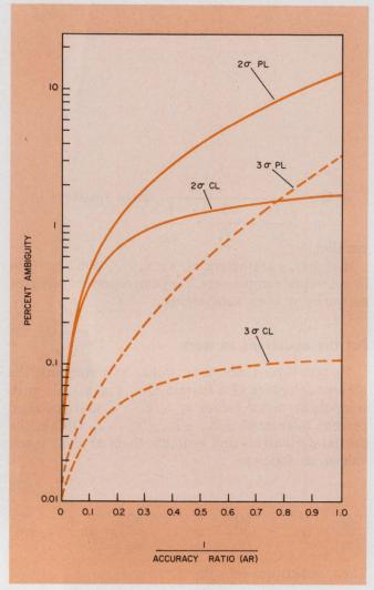
2. In this risk-assessment graph, the consumer loss (CL) or producer loss (PL), each expressed in percent, depends on the system's over-all accuracy ratio (AR) and the quality of the components as measured by the number of standard deviations,  $k\sigma_i$ , that the component limits,  $\pm T_{\mu_i} \mu_i$  are spread over.
