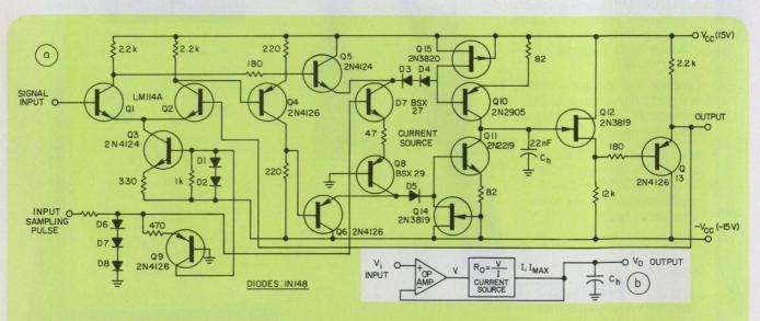
1. This sample-and-hold circuit (a) provides an overall accuracy better than 0.01% with a voltage droop
