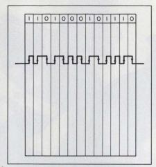
"Phase-encoded recording solved the problem. At every bit time, at least one flux reversal occurs—one reversal indicates a ZERO, two reversals indicate a ONE. The flux reversal is in one direction for a ZERO, another for a ONE. This scheme provides a self-clocking mechanism that can track a string of repetitive bits, no matter how long it is."
