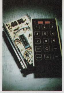
By bringing down the cost of microprocessors, General Instrument has been able to design them into costconscious items such as this microwave oven controller.
