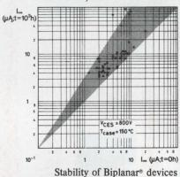
with  $V_{CBO} = 800$  V,  $V_{CEO} = 450$  V,  $I_{C} = 10$  A,  $P_{tot} = 125$  W, TO-3 metal case. The diagram demonstrates the stability of Biplanar® devices, with  $I_{CES}$  remaining constant before and after the 1000-hour life test at high voltage and high temperature.
