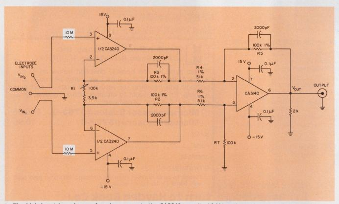
1. The high input impedance of each op amp in the CA3240 permits  $10\text{-M}\Omega$  resistors in the probe circuits.
