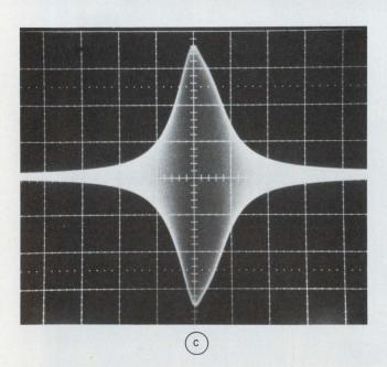
4. **BIFETs ensure stable operation at 100 kHz** for this cascade of two positive-feedback bandpass filter sections (a). The Q of 30 and the gain of 4 for each section (b) compound into a Q of 69 and a gain of 16 (c).
