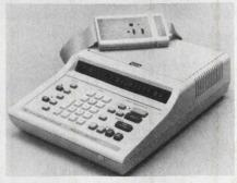
When a bus stops, the source of the failure must be found. Hooked up to the 1602A logic analyzer, this special probe from HP helps engineers visualize problems on the standard instrument interface.
