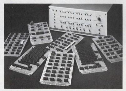
Low-cost PCM microcomputer modules offer full TTL bus compatibility, a variety of static and non-volatile memory modules expandable to 32K words, and a wide selection of I/O interfaces. Ask for complete product information.
