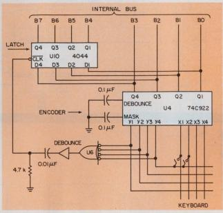
2. The internal bus, B<sub>0</sub> to B<sub>7</sub>, is the source of data and addresses while the memory is being loaded.
