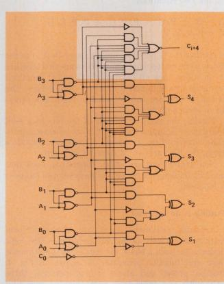
3. Improve the 4-bit adder with a carry-lookahead feature. The upper block implements the auxiliary function, while the lower blocks generate the sum bits.
