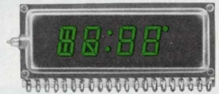
FG48D6 Dimension: 25.5(H)×56.5(W)×7(D)mm Character Size: 8.0(H)×4.2(W)mm
