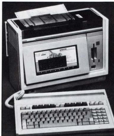
storage. A 25-lb unit 13 in. wide, 16 in. high, and 7 in. deep, it includes a 9-in. electroluminescent display driven by a proprietary
