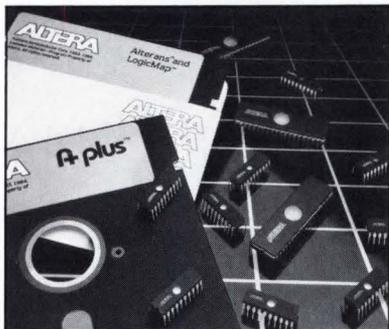
Written in C for easy portability, A + Plus allows users of erasable programmable logic devices (EPLDs) to enter designs using logic schematics. Other input formats include interactive net lists, state diagrams, and traditional Boolean equations. A + Plus runs on the IBM PC and PC-compatible computers, and it is compatible with third-party programmers such as Data I/O and Stag machines.
