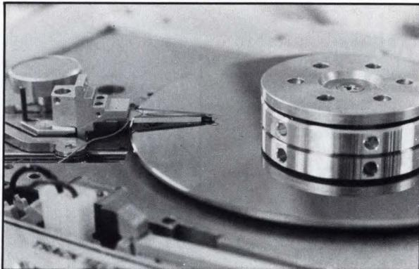
**A** series of thin-film read/write heads is one of the first to meet the needs of advanced hard-disk drives having densities in excess of 1200 tpi. The 1200 series, an addition to Read-Rite's RR-1212 line, will handle a data track width as thin as 250  $\mu\text{in.}$
