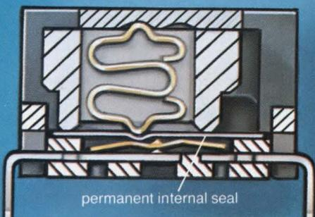
Exclusive internal seal protects gold-plated contacts during pc board production, test, and rework, and for the life of the switch.
