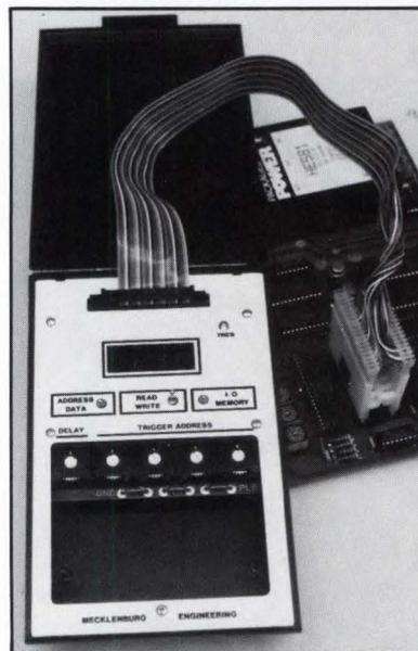
**P**ackaged in the form of a breakout box, a microprocessor bus-monitoring instrument is a useful debugging aid for real-time control software, since it does not affect the operation of the system under test. The Model 08 is available for use with a variety of 8-bit microprocessors. With some additional parts, the system can be easily reconfigured to accommodate 6502, 6809, 8085, and Z80 devices.
