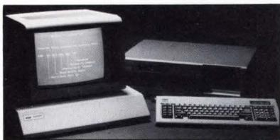
The base unit—a self-contained 8088-based single-board computer—has eight digital inputs, four digital outputs, and four analog inputs, plus four connectors to accommodate additional I/O modules. Up to 255 Series 10 units may be separately addressed in a single system.
