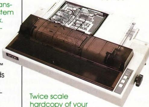
Twice scale hardcopy of your artwork is produced using the Epson dot-matrix printers or the Houston Instrument DMP-41 pen-and-ink plotter. Quick 1X check plot is also available from Epson printers.
