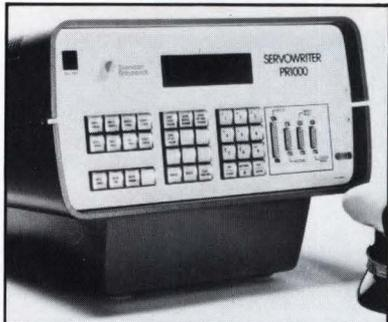
**W**ell suited for R&D, production, and depot service applications, the PR1000 writes Winchester servo tracks without the use of a mechanical positioner, granite blocks, lasers, or other accessories. The portable unit cuts the cost of a full-blown servo writer from over \$250,000 to under \$50,000. Furthermore, the PR1000 servo writer is fully programmable and does not require costly reconfiguration to handle different sets of drive characteristics.
