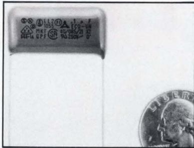
**D**esignated the ECQ-UN series, a family of metalized-film capacitors is approved by most international standards agencies, including UL, CSA, VDE, SEMKO, and SEV. The universal capacitors are suitable for across-the-line applications meeting UL/CSA standards and class X applica-
