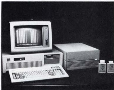
Costing less than most stand-alone logic analyzers, the MicroAnalyst workstation integrates the power of an IBM PC AT with the Series 2000 logic analyzer and a Lotus-based general-purpose software package. Five software functions—spreadsheet, data base, word processing, graphics, and communications—allow the user to perform complex data analysis.
