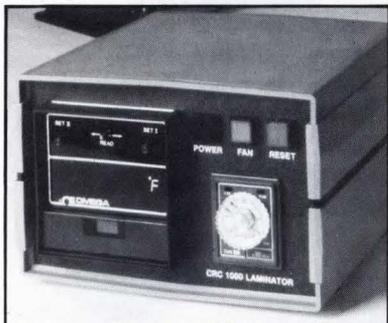
The CRC 1000 gold contact laminating system adds or replaces gold finger contacts on printed circuit boards. Production yields are increased by repairing rejects, and full restoration of traces marred by scratches, corrosion, pits, or voids is accomplished by the lamination of new, precisely etched, polyimide adhesive-backed replacement contacts.
