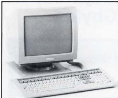
**P**riced nearly 40% lower than the DEC VT220, the TVT-7220 video terminal offers 100% emulation of the DEC unit. Quantity shipments of the TVT-7220, which carries a suggested retail price of \$850, are available immediately. The terminal has a 14-in. display, a tilt-and-swivel enclosure, and a 105-key DIN-standard keyboard. The display screen can be formatted for 80 or 132 columns. In addition to full emulation of the VT220, the TVT-7220 emulates the VT100 and VT52 terminals.
