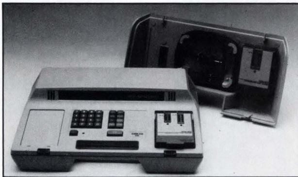
**A** universal programmer allows an engineer to program over 99% of all existing programmable logic devices, including PROMs and PAL and IFL (integrated fuse logic) devices. The Model 60A, made by Data I/O, is available with a handler interface for programming parts in production quantities.
