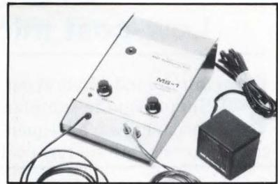
create an ac magnetic field in the vicinity of the shorted current path. The MS-1's Omni-Probe responds to any orientation of the resulting three-dimensional flux patterns and emits an audible tone whenever it is held near a 300-kHz current-carrying conductor. Faults are typically located in less than one minute.
