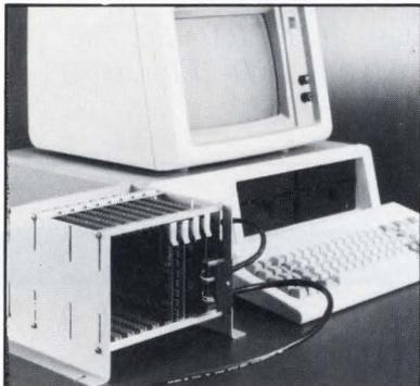
**B**ased on the WD2840 LAN controller chip, a LAN interface card connects the IBM PC with the STD bus for industrial control applications. The card, designated the NETPC/STD, implements a token bus protocol that is similar to Arcnet, but with higher throughput rates (1 Mbit/s) and greater noise immunity. Lengths of up to 1000 ft between daisy-chained nodes are permitted, with a maximum total distance of 10,000 ft.
