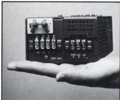
To enhance reliability, the LR series of fifth-generation switching power supplies incorporates a custom integrated control circuit that replaces 40 discrete components. The 16 models that comprise the LR series provide adjustable fixed voltages of 5 to 48 V. Current ratings include up to 40 A for the lowest-voltage supply and up to 5.8 A for the highest-voltage supply. Ripple is from 10 to 35 mV, depending on the output voltage. Line and load regulation are 0.1%.
