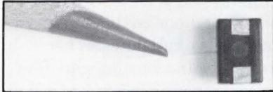
In keeping with the trend toward miniaturization, the MKT 1824 metallized-film chip capacitor comes in three sizes with maximum lengths of 4.2, 5.7, and 7.5 mm. All three sizes are rated for 63 V dc. Capacitance values range from 0.01 to 0.15  $\mu\text{F}$  for the 4.2- and 5.7-mm-long devices and from 0.01 to 0.22  $\mu\text{F}$  for the 7.5-mm-long chip. The MKT 1824 capacitor is suitable for wave soldering up to 260°C (for 5 seconds) and reflow soldering up to 260°C (for 10 seconds).
