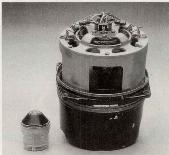
2. A TYPICAL GYROSCOPE used in military aircraft (right) weighs about 5 lb. and is 5 in. wide by 8 in. high. In contrast, the GyroEngine (left) is about the size of a roll of film. Five electrical contacts on the top of the GyroEngine provide power to the unit: two for power to the gyro motor, and three for torque voltage, which corrects for gyro precession.
