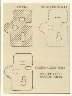
**Figure 3**—Vectorization is performed on image data previous to its being classified.
