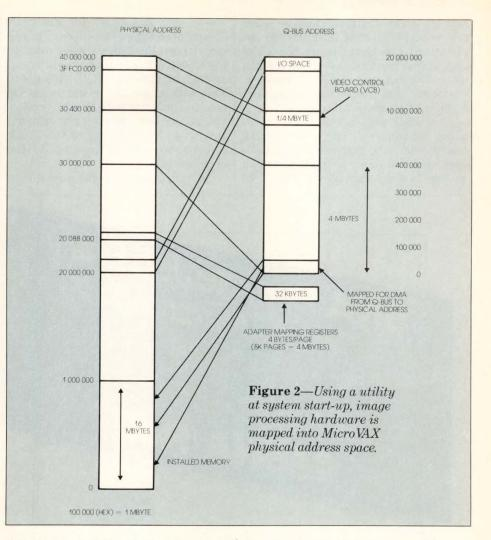
this frame buffer section be large enough to allow one frame buffer (512 Kbytes) to be mapped at once. A utility can do the work of creating these globals and inform VMS of the board's presence, and allowing users access to the board as a system resource. These sections are referenced by name and the user process must map them into its virtual address space.
