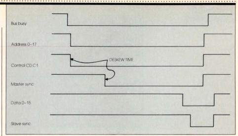
**Figure 2**—*The Unibus waits a de-skew time of 150-180 nsec for the bus to settle down before asserting the master sync signal to notify all devices on the bus that a command is waiting for the slave identified by the address.*
