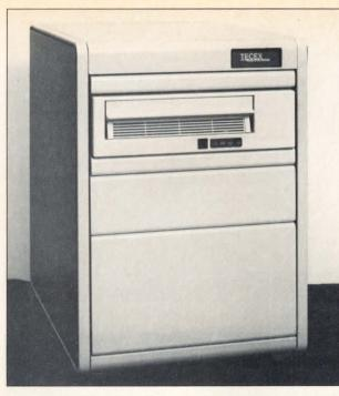
U.S. Design Corp. also offers optical disk products for the Digital environment. Its 1108 (Q-bus) and 1158 (Unibus) SCSI host adapters have been firmware "tailored" for support of all major manufacturers of optical disk drives, including OSI, Sony, Hitachi, Figure 1—The TEC-OAS/1 Optical Archiving Subsystem for VAX architectures from the Q-bus to the Unibus was configured by TECEX.
