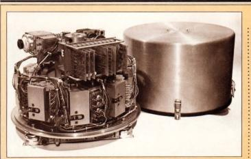
**Highly reliable but out-of-date**—*Drum storage devices implemented a separate read/write head for every data track.*
