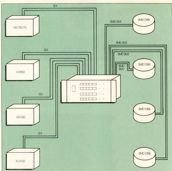
disk controller that supports SDI, including the HSC50/70 used on VAXclusters and the KDB50 used on VAXBI systems.
