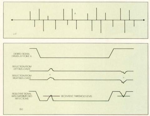
**Figure 9**—A complex stub layout (a) is the reality behind an actual system bus. These stubs have a substantial effect on bus signals (b).
