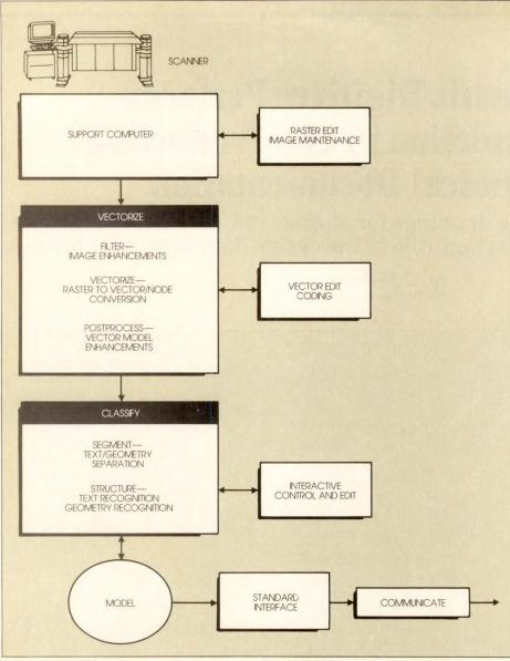
**Figure 2**—When an image is automatically digitized, it is first scanned, then vectorized. Next it is reduced to its component parts and the intelligent output model is produced.
