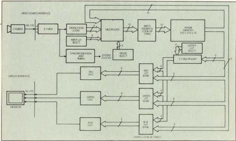
**Figure 1**—*Image processing hardware for the MicroVAX II can be integrated onto a single board.*
