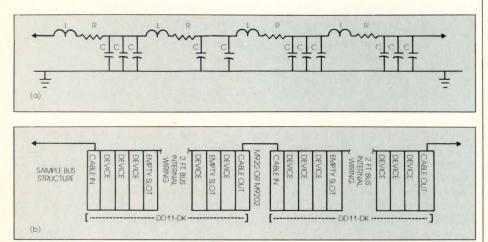
**Figure** 8—The electrical representation (a) of a sample system bus structure (b) shows the complex RLC make-up of an actual system bus.
