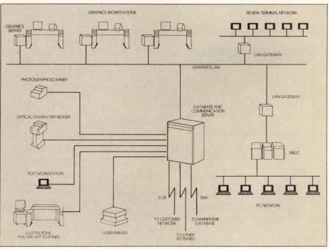
**Figure 1**—A typical system configuration for the automation of technical documentation enables review, revision, and composition of both graphics and text data, as well as the storing and distribution of it.
