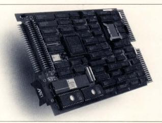
Figure 1—MTI's MSV15 TSV05/ TS11 compatible ½in. tape coupler for the Q-bus is an example of the new dual-wide high performance tape control boards.
