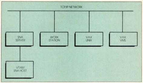
Figure 1—An SNA server links a TCP/IP network to a host using SNA. Using an API, a software bridge is created that provides UNIX or VMS access to SNA host data.
