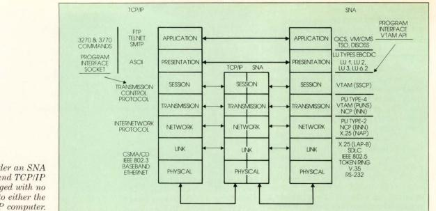
Figure 2—Under an SNA LAN, SNA and TCP/IP are bridged with no modifications to either the IBM or TCP/IP computer.
