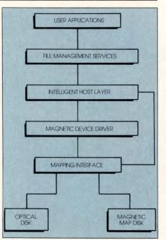
**Figure 3**—The magnetic mapping for optical disk concept implements an intelligent layer that defines multiple write intervals to an associated mapping interface.
