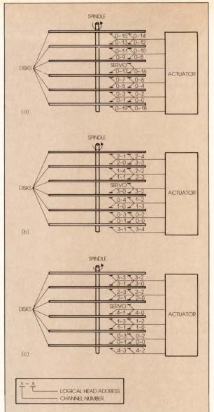
M2360A disk drive, for example, there are six 10<sup>1/2</sup>-in. platters and two heads for each of the 10 data surfaces—the top surface isn't used and one other surface is reserved for prerecorded continuous servo information (the servo surface has its own head). The high storage density of the drive (18,620 bits/in. linear density and 880 tracks/ in. areal density) magnifies every tracking error, so continuous closedloop servo tracking is imperative.
