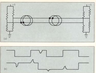
Figure 6— Crosstalk occurs when lines of flux cut across conductors (a). The resulting waveform shapes in the conductors are distorted (b).
