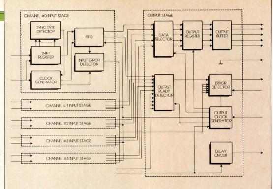
Figure 3—De-skew circuitry eliminates data timing synchronization problems between channels that arise due to electrical or mechanical variances.
