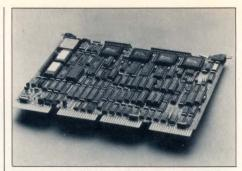
**Figure 3**—SMS's SMS0108 is a triplefunction (Winchester, floppy, QIC-02 ¼in. tape) TMSCP controller that represents a trend in highly integrated multifunction controllers.
