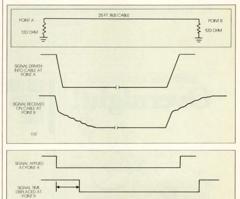
**Figure 3**—Due to high frequency cable loss, the quality of the digital signals on the Unibus deteriorates as the signal moves through the cable (a). Propagation delay is another problem, and is defined as the difference in time between when a signal occurs and when it is received by the affected component (b).
