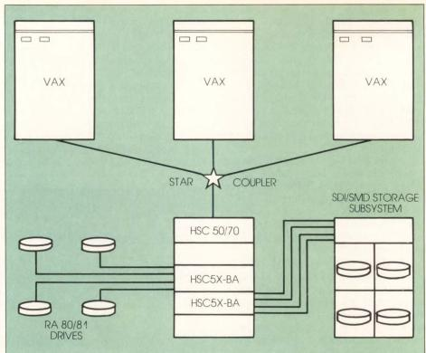
Figure 2—In an existing VAXcluster installation, SDI/SMD storage subsystems can be added to, or mixed with, existing RA80/81 drives.
