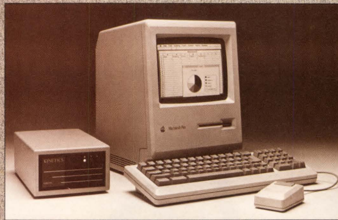
The Kinetics EtherSC directly connects a Macintosh to Ethernet.
