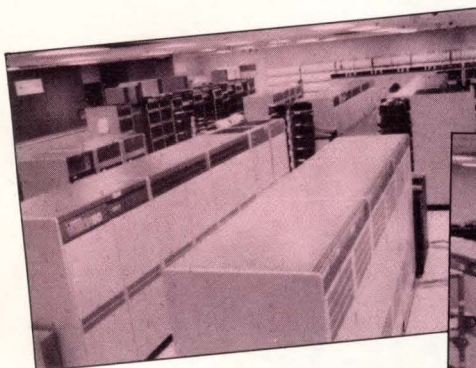
DECsystems galore —CompuServe hardware includes 43 DECsystems and one Systems Concepts mainframe.
