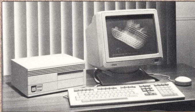
The monochrome VAXstation 2000 workstation offers CPU performance equal to a MicroVAX II system, but fits easily on a desk.
