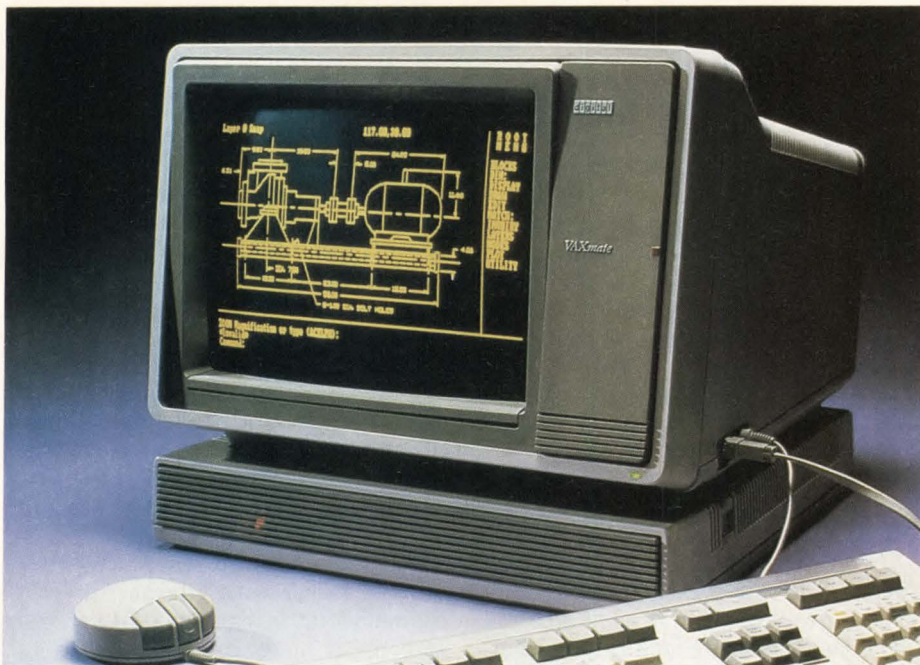
Figure 2 —To execute VAX/VMS graphics applications using the VAXmate as a graphics terminal required the video control and monitor be designed to have an 800 x 240 mode of operation. The VAXmate video actually has an 800 x 250 mode of operation.
