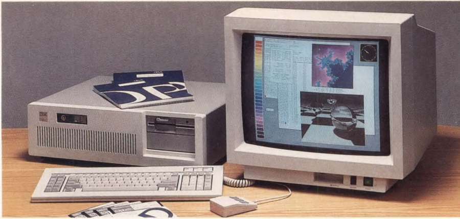
Figure 1 —Although it's possible to run X Windows in color, as depicted, with the proper interface card, the HC/WG Labs workstation used a Moniterm Viking 1 monochrome display. Either way, X Windows provides a high-level graphics interface that provides the same windowing system used by Apollo, Data General, DEC, Hewlett-Packard, Siemens, and Sun Microsystems in their workstation systems.
