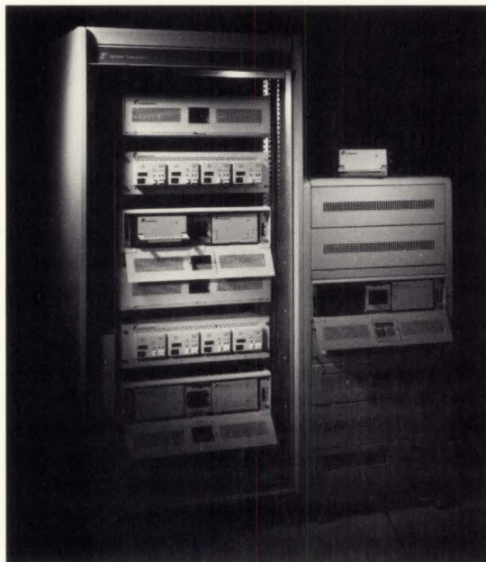
Figure 3—The disk units used in System Industries Inc.'s (SI's) 5.25-in. Quick Disconnect Systems are interchangeable among all SI 5.25-in. quick-disconnect carrier slots. A flush-mounted handle is integrated into each drive's faceplate for easy transport, but a two-step powering-down procedure prevents accidental removal.
