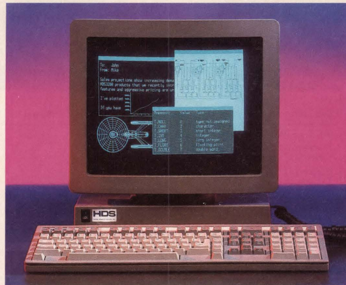
With a price tag of $1,200, Human Designed Systems Inc.'s HDS3200 Model 30 Image Leader monochrome terminal provides affordable 1056 x 800 resolution for a wide variety of graphics applications.
