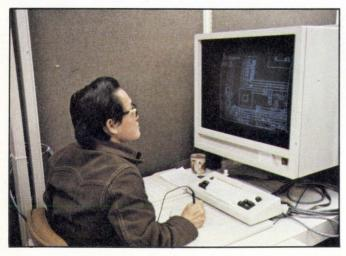
**Designer Cahi Un Tak** uses applications graphics terminal to lay out section of VLSI circuit. He locates circuit elements, then transfers section to a DEC VAX-11/780 supermini for design-rule and continuity checking.
