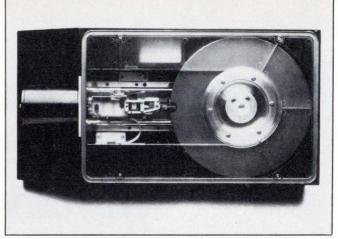
Fig. 3. Multi-platter, fixed, 8-in. drives such as this 6170 series unit from BASF boast large capacities. The unit above stores 40M bytes on three platters and uses a linear actuator to achieve 27-msec. average head-positioning times. The 6170 is driven by a DC motor, has a 10,000-hour MTBF and does not require scheduled maintenance
