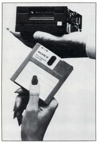
Fig. 3. Sony's  $3\frac{1}{2}$ -in. Micro Floppy disk stores 437.5K bytes per disk and measures  $2 \times 4 \times 5.1$  in. For word-processing, personal and business applications, the drive uses a video-type precision head.
