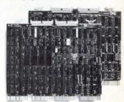
Q-bus embedded dual-density tape controller.
