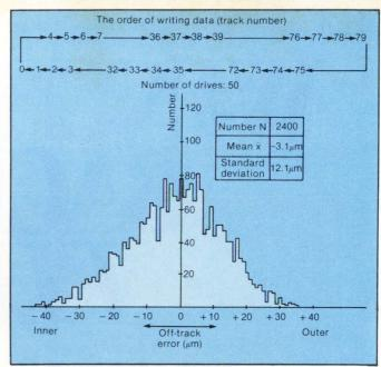
Fig. 4. Positioning accuracy test results for the YD-280 show that Y-E Data surpasses its  $\pm 5$ - $\mu m$ . off-track error specification. Precise electromechanical components and careful assembly produce an average off-track error of  $-3.1~\mu m$ . for 2400 track samples. While all errors were within the  $\pm 50$ - $\mu m$ . range, the majority were within 12.1  $\mu m$ . of the track center.
