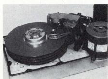
ter-disk drive offers SMD interfacing, a closed-loop track-following positioning system and a rotary voice-coil positioner. The unit has a 11,500-bpi bit density, a 600-tpi track density and a 45-msec. average access time. Other features include self diagnostics, a Z80A  $\mu p$  and 3600-rpm spindle speed. **SLI Industries**, 21040 Victory Blvd., Woodland Hills, Calif. 91367.
