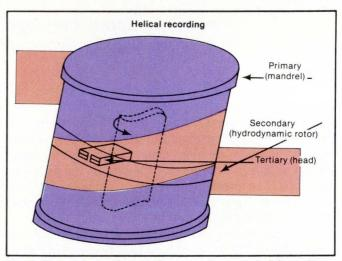
Fig. 3. Helical recording devices use the mandrel for primary stability, and hydrostatic forces between tape and rotor provide secondary stability. Tertiary stability, as with linear devices, is created by the air bearing between head and tape. The spindle turns the rotor and heads.
