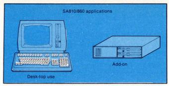
Shugart's SA810/860 half-height, reduced-depth 8-in. floppy-disk drives give a system designer the flexibility of placing the drives within the terminal or as add-ons.
