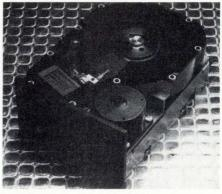
μp. The device offers a 130-msec. average access time, a 3-msec. track-to-track access time and a 5M-bps data-transfer rate. Other features include step-pulse buffering, head-velocity profile control and off-track positioning. Computer Memories, Inc., 9233 Eton Ave., Chatsworth, Calif. 91311.
