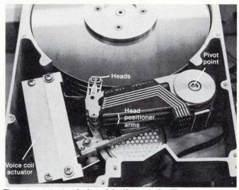
The rotary actuator design of the Kennedy PosiTrack, in which the voice coil actuator is only 2 in. from the heads, achieves high precision and stability. The unit sells for \$2240 each in OEM quantities.
