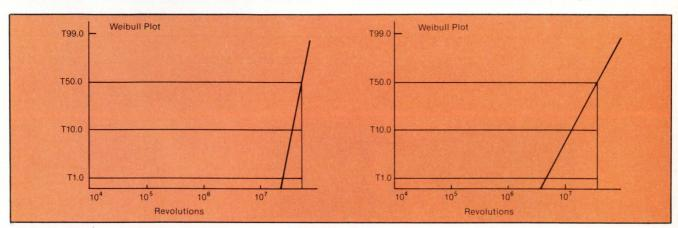
Fig. 1. Durability predictions in terms of how many failure-free revolutions can be expected from 1 percent, 10 percent, 50 percent and 99 percent of a disk sampling are more meaningful than those that tell only median failure time (T50). For example, although both Weibull plots above show the same T50, the sloping durability line of the plot at left indicates more consistent results than that of the plot at right.
