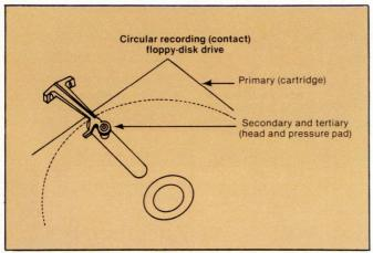
Fig. 4. The floppy-disk establishes primary stabilization via its jacket, which is also an immediate cause of wear. The head/pressure-pad combination provides both secondary and tertiary stabilization.
