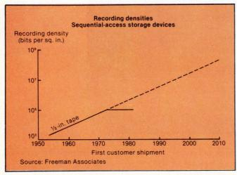
Fig. 2. IBM's long-awaited announcement of new drives using higher track and bit densities on ½-in. tape is expected to trigger several competitive responses and move tape-recording densities ahead toward this projection.
