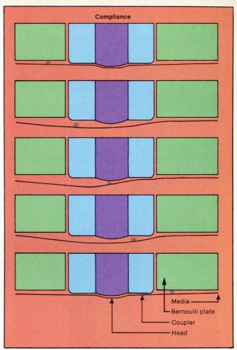
Fig. 8. As a particle on the medium approaches the coupler (top), an inrush of air breaks the coupling, and the medium pulls away, or "compiles." This permits the particle to traverse the head-coupling region without making contact with the head. Coupling is then reestablished, leaving only a read or write soft (non-repeatable) error.
