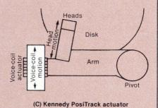
A comparison of rotary-actuator designs shows that the Kennedy PosiTrack situations the voice-coil actuator closer to the read/write head. This results in improved head positioning and tracking, as well as lower susceptibility to shock and vibration.
