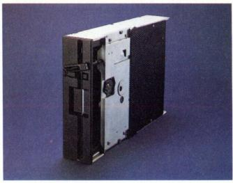
Shugart's SA810/860 8-in. floppy-disk drives are 2.31 in. high, exactly half the height of standard-sized floppies, and are only 12 in. deep, the same depth as a CRT terminal. The SA810/860 is shown with optional metal shields (r.), which protect against external EMI sources such as CRT flyback transformers or switching power supplies that often are next to disk drives.
