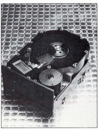
Fig. 5. Rising 51/4-in. disk capacities are exemplified by this 19.14M-byte unit from Computer Memories, Inc. Recording almost 5M bytes on each of its four platters, the model CM 5000 features Winchester technology, industry-standard mounting dimensions and optional transfer rate for 8-in. Winchester compatibility.
