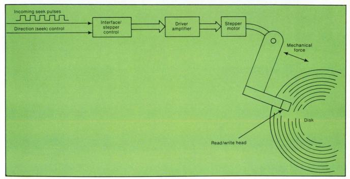
Fig. 1. Open-loop stepper systems receive seek commands from the disk's actuator-control circuitry. Receipt of one such pulse causes the head to move one track. The direction-control line determines the direction of seek motion. An interface/stepper controller converts the positioning signals to stepper-motor commands.
