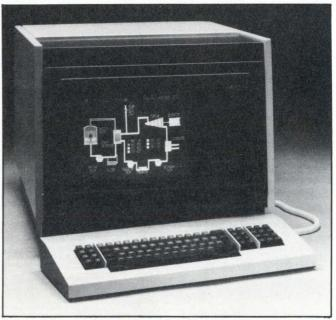
Colorgraphic Communications Corp.'s \$3500 Z80-based MVI 7 has a resolution of  $720 \times 280$  pixels and displays seven foreground and background colors.
