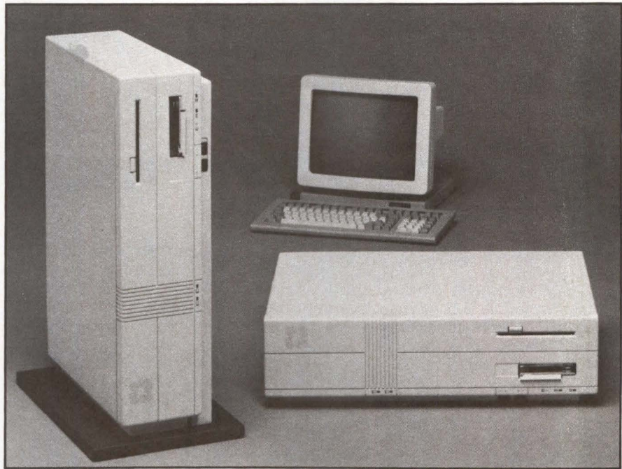
Rair's 80286-based SuperMicro computer comes in a floor-standing (left) or desktop configuration.
