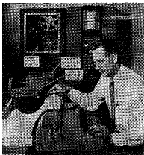
Fig. 6—Computer, magnetic-tape unit, and input-output unit.
