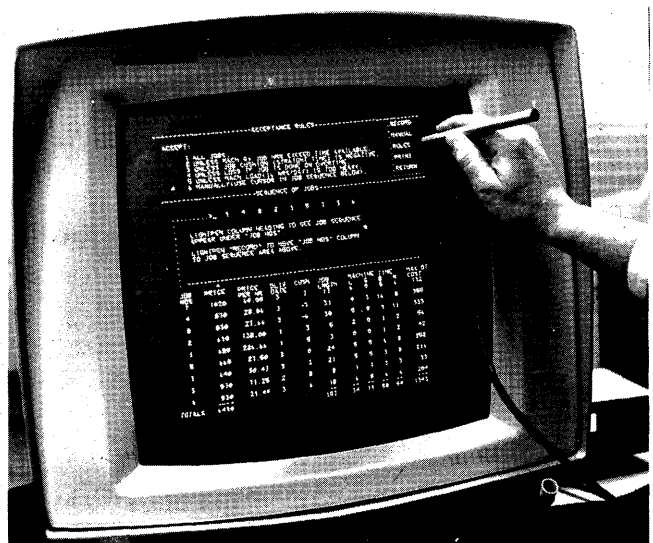
Figure 6—Supplementary information panel to assist scheduler in making acceptance and sequencing decisions
