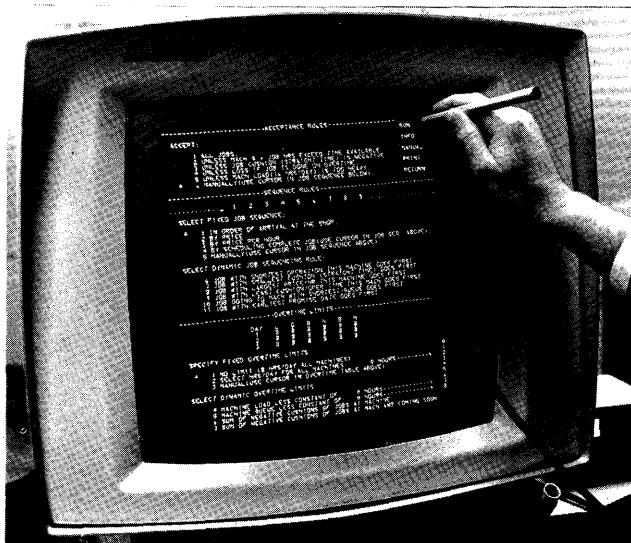
Figure 1—Decision rules for job shop scheduler, selected by light pen at IBM 2250 display unit
