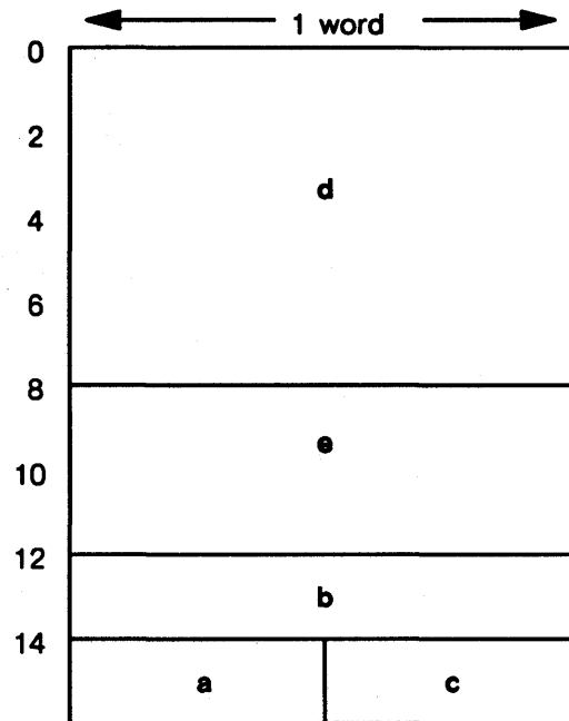
Figure 3-13. Memory Arrangement According to Decreasing Size of Fields
