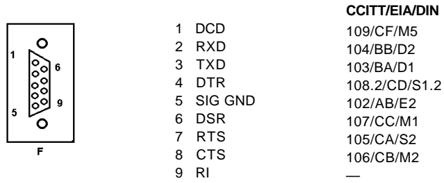
Figure A-2 9-Pin EIA 232 Port
