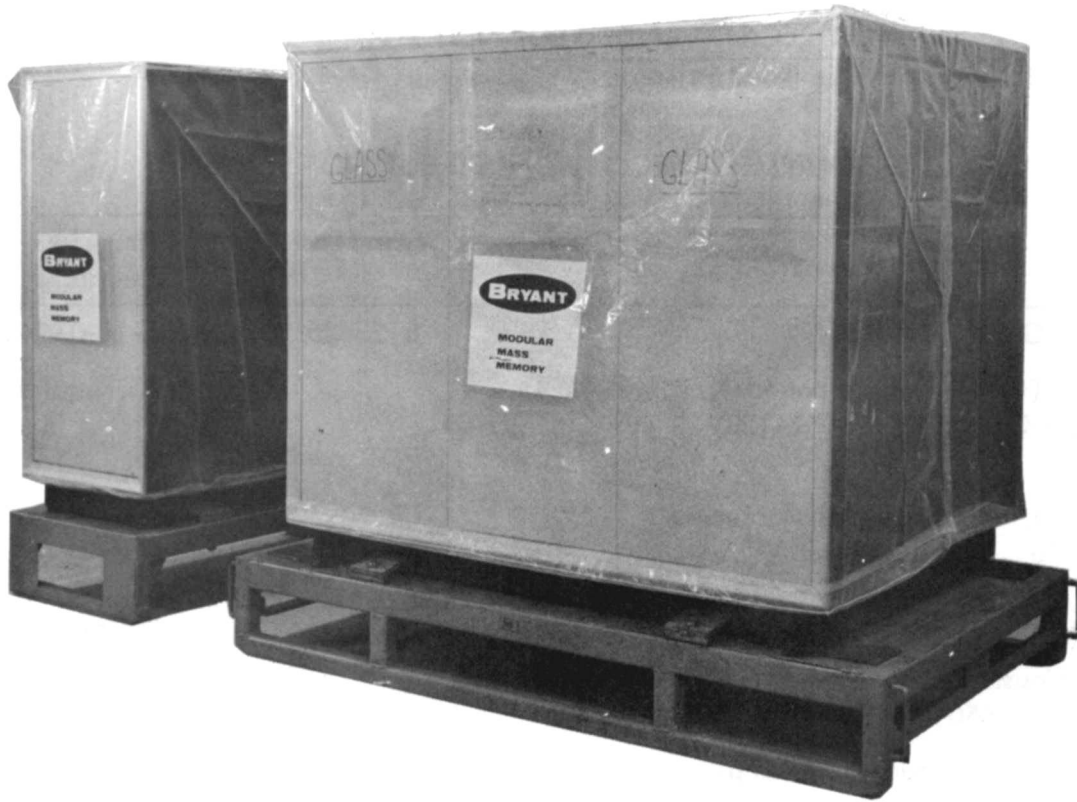
Figure 2-1 Model 1 Series 4000B Disc File Sealed for Shipment—Typical Sealing of All Files
