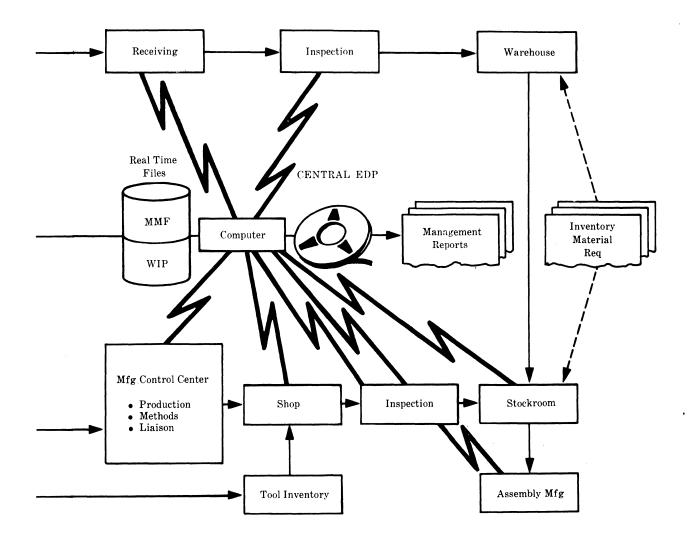
basis for central electronic data processing. When the part reaches the stockroom, up-to-theminute information is used to update computerized ship coverage records. About 80,000 work orders of an average of 20 pieces each are tracked. The real-time feature of MIS allows immediate remedial action for situations such as tool and material shortages on the shop floor and configuration discrepancies. The shop tracking data collection system can handle up to 36,000 transactions per hour.
