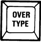
**OVERTYPE** causes the letter at the cursor position to be replaced by the one just entered. Normally, the keyboard is in "insert" mode, where new letters cause existing letters to shift to the right at the cursor position.
