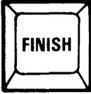
**FINISH** ends a command operation or an applications program. In the BTOS command line you would use **FINISH** to stop further operation of a command. In many applications programs, **FINISH** signals your request to stop the current work session.
