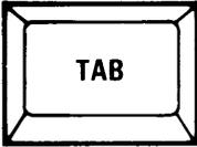
**TAB** moves the cursor to a tab stop that has been set within an applications program. Within the BTOS command line (shown in Section 1), it moves the cursor to the next line on the screen.
