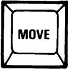
**MOVE** is not used for operations in the BTOS command line. It functions within word-processing programs such as the BTOS Editor or the Professional Word Processor program.
