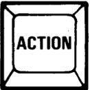
**ACTION** is always used in conjunction with another key. For example, pressing **ACTION** and **OVERTYPE** simultaneously clears the screen of your monitor. Pressing any key restores the screen to its full display.
