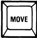
**MOVE** is not used during operations within the BTOS command line. It functions within word-processing programs such as the BTOS Editor.
