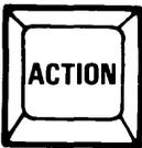
**ACTION** is always used in conjunction with another key. For example, pressing **ACTION** and **OVERTYPE** simultaneously clears the screen of your monitor. Pressing any key restores the screen to its full display.
