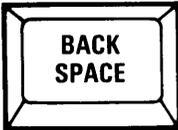
**BACK SPACE** allows you to delete the previously entered letter. If you hold the **BACK SPACE** key down, it deletes letters continuously. With **OVERTYPE** on (see Control Keys), this key does not delete letters but moves the cursor one horizontal position to the left.
