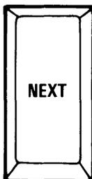
**NEXT** re-positions the cursor at the beginning of the next line on the screen. It is located with the number keys for ease of use when you are entering numbers.
