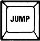
You press **JUMP** to move the cursor to a new position. The new position is defined by a Text Segment Key (for example, **LINE** or **PAGE**).
