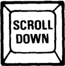
**SCROLL DOWN** causes a line of new information to be added to the top of the screen. It does not function within the BTOS command line, but is very important for many applications programs, such as word processing.
