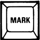
**MARK** is not used for operations in the BTOS command line. It specifies the beginning of a word or group of characters to be changed (moved, deleted, copied, and so on) within a word processed document.
