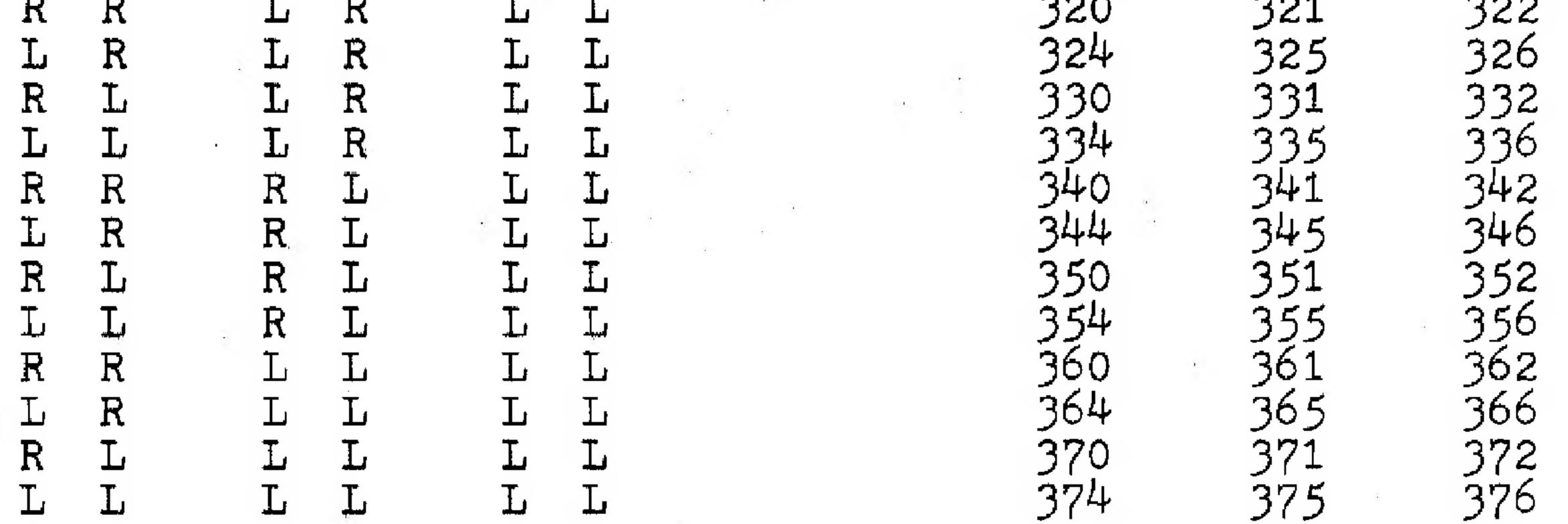
\* For compatibility with Cromemco software we recommend this port assignment: Port A - 020; Port B - 021; Port C - 022. For this port assignment connect the address selection jumper wires as shown in this diagram:
