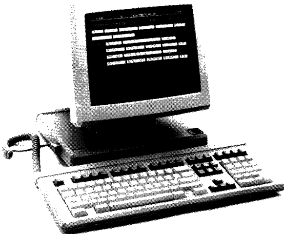
The Falco 5500 is a high-end ASCII terminal, featuring a high resolution screen and multi-host windowing.
