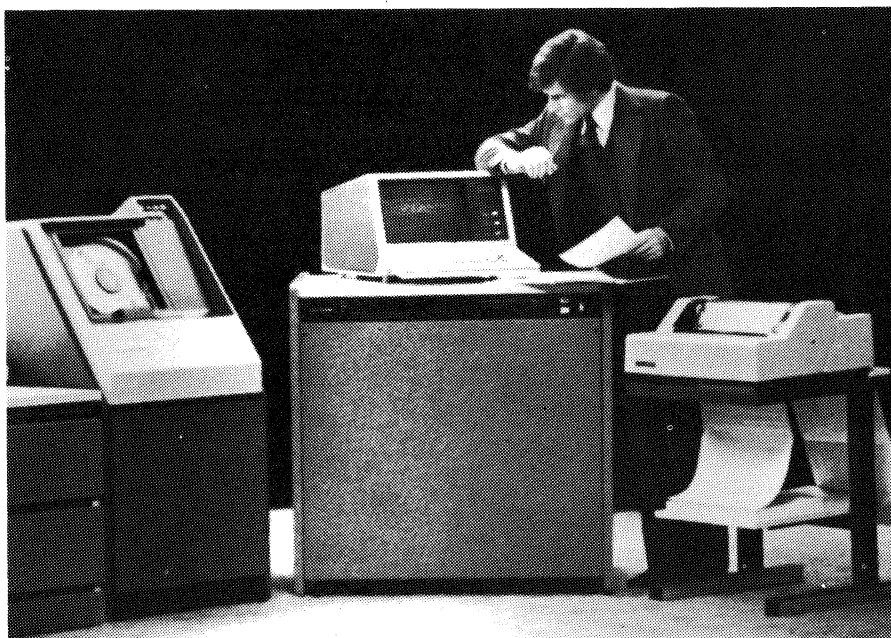
The DCP/20 Processor (center) is shown in configuration with (from left to right) the cartridge disk sub-system, one Uniservo 10 tape drive, and the optional operator's control console and impact console printer.
