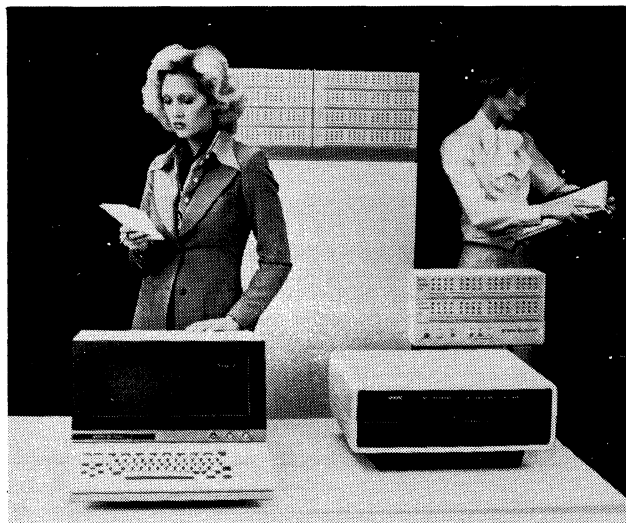
In the foreground is a UNISCOPE 100 Console and a diskette unit atop the Distributed Communications Processor's desk-like cabinet. In the background is the Type II Scanner.
