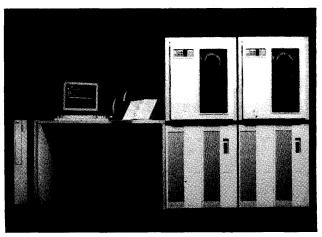
The high-end Model 8 of the ADDS Mentor 6000 supermicro supports from 4MB to 16MB of memory and can handle up to 160 users. Disk capacity ranges from 534MB to 3.5GB of storage.
