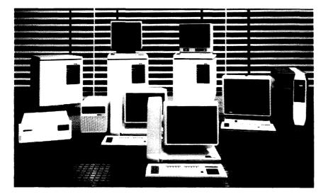
The Apollo Domain Systems are compatible 32-bit computers that feature high-resolution, bit-mapped graphics, and operate in a distributed local area network. The DN550 is a mid-range color workstation that supports up to 3MB of memory and 1.05GB of disk storage.
