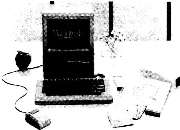
*Equipped with Motorola's 16-/32-bit MC68000 microprocessor chip, the Macintosh includes 128K bytes of main memory, 64K bytes of ROM (which contains the operating system), an integral 9-inch screen and 3½-inch microdiskette drive, detached keyboard, mouse, learning manuals, and audio cassette. With the addition of a keyboard, mouse, manuals, and carrying case, the Macintosh weighs in at 23 lb. but its footprint is smaller than an 8½-inch by 11-inch sheet of paper.*
