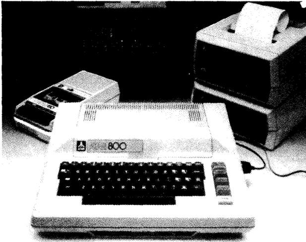
The Atari 800 shown here consists of a 16KB RAM, cassette program recorder, 40-cps 4-inch roll printer, 5 1/4-inch 88KB mini-diskette drive, and a user-supplied color TV set or monitor. Programs can be loaded either via plug-in ROM cartridges, cassette tapes, or diskettes. The 800 is programmable in Basic or Assembly language.
