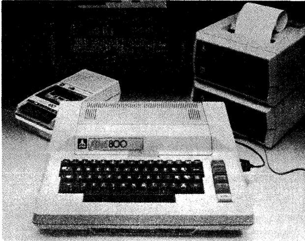
The Atari 800 shown here consists of a 24KB RAM, cassette program recorder, 600 lpm 4-inch roll printer, 5/4-inch mini diskette drive capable of storing up to 92KB, and a user supplied color TV set. Total cost of this system is about \$2,500. Programs can be loaded either via plug-in ROM cartridges, or on cassette tapes. The 800 is programmable in BASIC or Assembler language.
