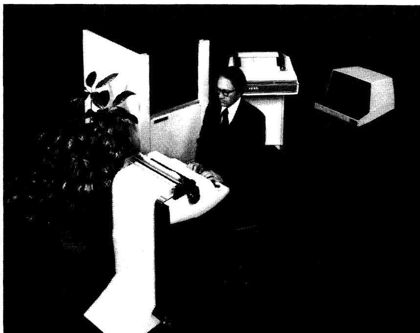
The BTI 5000 is shown with the optional Model 5620 (300 lpm) line printer to the right of the processor cabinet. The terminals shown are examples of units frequently used with the 5000. Terminals are not included in BTI's product offerings.
