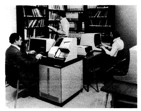
This top-of-the-line Cyber 18-30 utilizes two processors (one for time-sharing, the other for communications) while supporting up to 64 interactive terminals. Oriented toward educational institutions, the 18-30 can be configured with a maximum of 400 million bytes of disk storage and up to 512K bytes of shared main storage.
