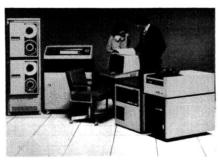
The Cyber 18-20 features a memory size of from 32K to 256K bytes, 9 I/O slots that accept magnetic tape, floppy and hard disks, a card reader/line printer, and micro memory controllers. A typical 18-20 system with 192K bytes of memory, ten terminals, 300 lpm printer, and 100 megabytes of disk storage costs about \$115,000.
