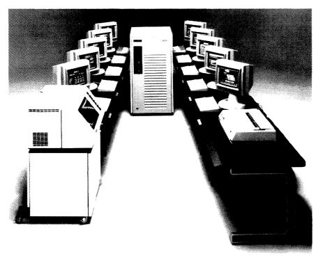
The Tiger ATS 64, shown here, is built around a triprocessor architecture that supports up to eight Transaction Processors, one Control Bi-Processor, two Intranet Processors, and two Global Memory Modules. The ATS 64 can accomodate 568MB of storage via 30MB, 60MB, or 143MB hard disks.
