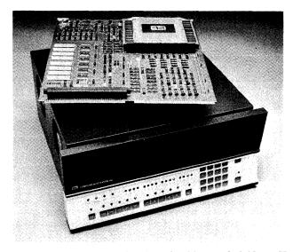
Fully compatible with each other, the 16-bit Naked Mini LSI 'computer on a board" (above) with 8K words of memory, and its companion, the fully clothed LSI with up to 72K words of memory (in the chassis), are the latest in CAI's line of OEM minicomputers. Both models implement LSI technology, a powerful instruction repertoire, and unique packaging schemes to offer an exciting product to the OEM minicomputer systems market.
