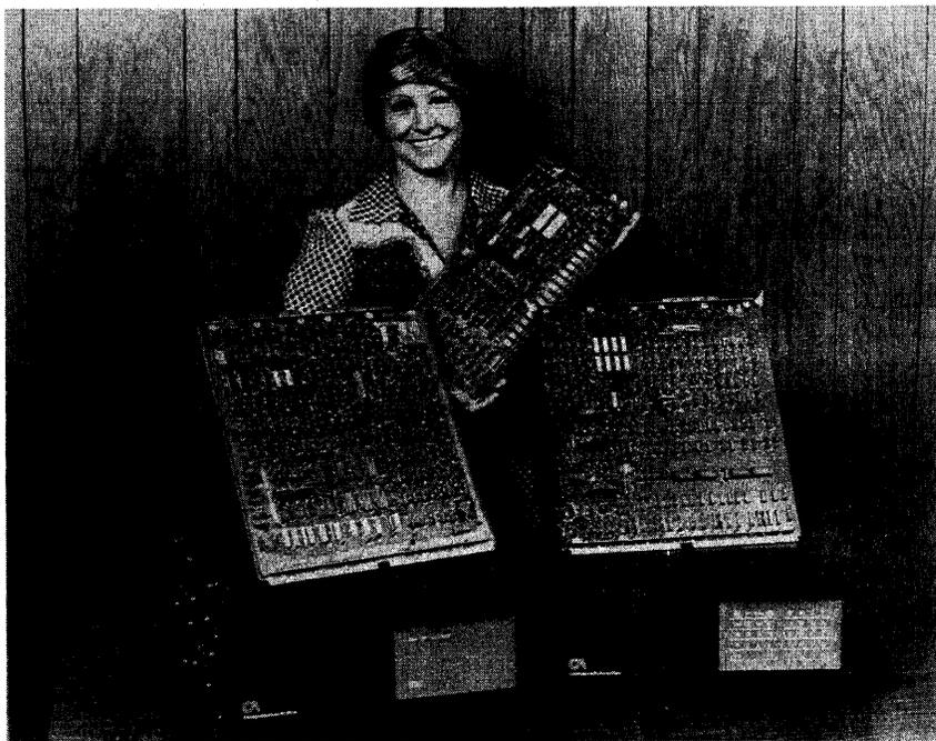
The LSI 4 family of processors includes the LSI 4/30, LSI 4/10, and LSI 4/90 (upper left to upper right). Packaged versions come in either an operator's console (lower left) or a programmer's console (lower right).
