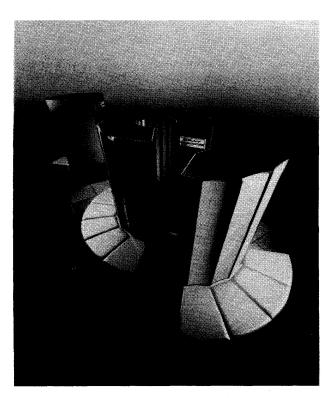
The X-MP/4 systems include 4 central processors with 64 or 128 megabytes of main memory. In this photograph, the mainframe is in the center. To the left is the I/O subsystem and to the right is a Solid-State Storage Device.
