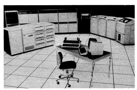
An enhanced DECSYSTEM-2060 has an improved price-performance capability. This system offers a new Intelligent Mass Storage Server, the HSC50, which will support high-performance disk and tape drives RA81, RA60, and TA78.
