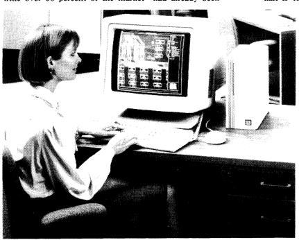
Digital Equipment Corporation's VAXstation 2000 is a desktop technical workstation designed for use in networked and clustered configurations, especially for technical computing in corporate environments. The workstation runs Digital's proprietary MicroVMS operating system and MicroVMS Workstation Software or the Unixderivative Ultrix-32m and Ultrix-32w workstation software.
