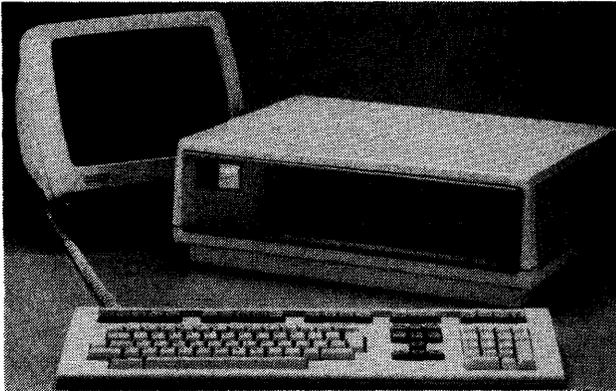
*The Rainbow 100 is a dual microprocessor-based personal computer that runs both 8-bit and 16-bit applications software under CP/M-80 and CP/M-86 as well as MS-DOS.*
