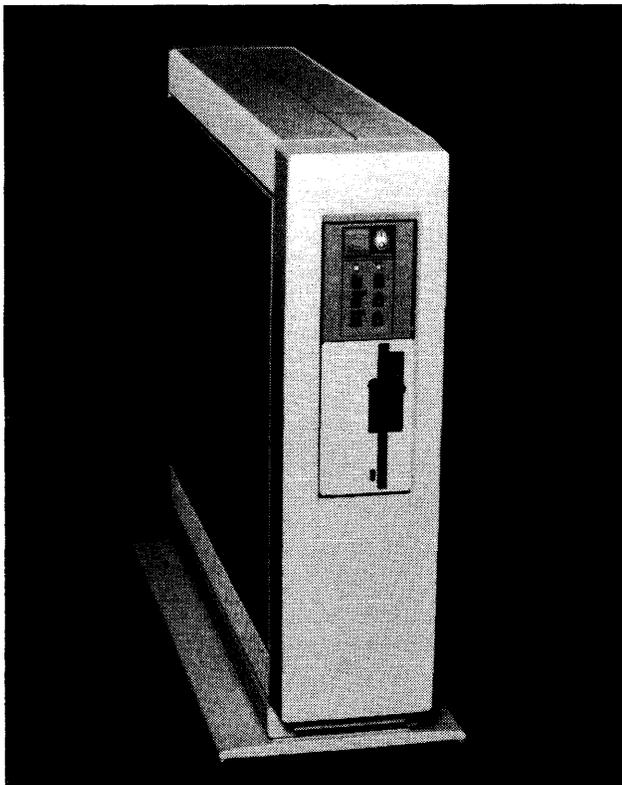
The MicroPDP-11/53 is typical of the downscaling that has occurred in the PDP-11 Family: the conventional minicomputers that used to comprise the product line have been repackaged as low-end multiuser microcomputers. The BA23 pedestal enclosure shown here is shared by MicroPDP-11, MicroVAX, and VAXstation systems.
