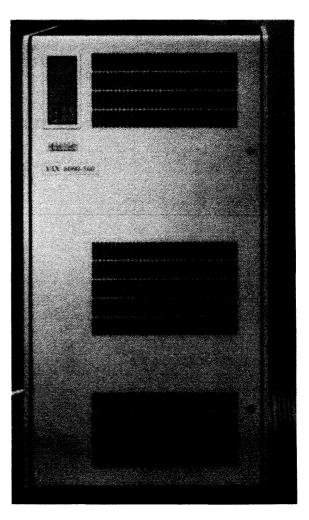
The VAX 6000 Series Model 500 offers enhancements in I/O performance, CPU performance, and memory and disk capacities. For departmental and data center computing, these new systems feature symmetric multiprocessing and a high-speed interconnect as a streamlined I/O path that provides three times the I/O throughput of earlier systems with the VAXBI bus.
